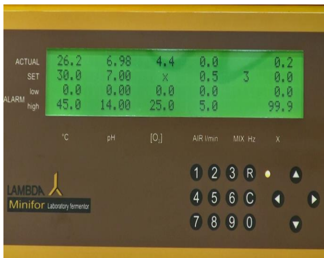
Figure 5.2—17 After pressing the regulation key "R", the MINIFOR changes to the standby mode from the Calibration mode.
