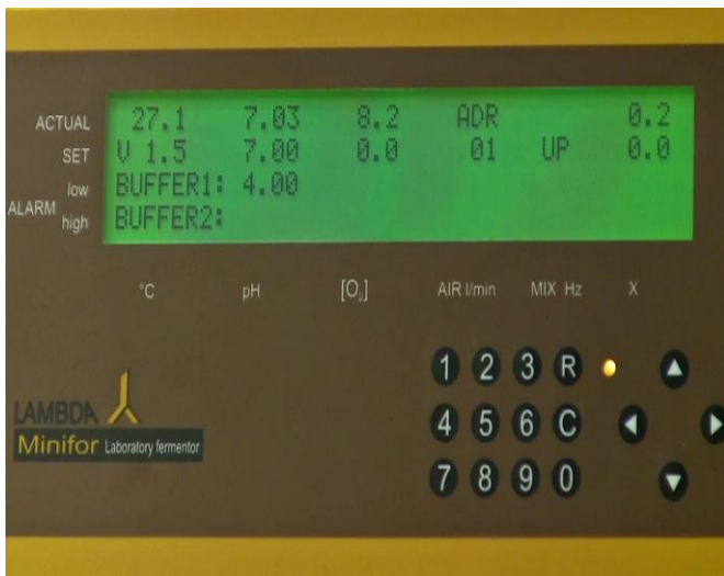
Figure 5.2—13 Wait until the ACTUAL value if the gauging solution becomes stable.
