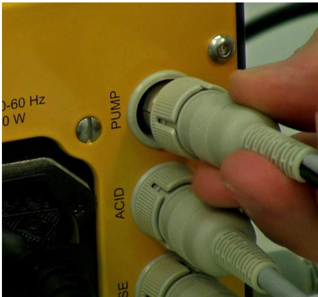
Figure 3.15—33 Connect the grey colour ANTIFO cable (8 poles) to the "PUMP" socket present on the rear of the MINIFOR base control unit.
