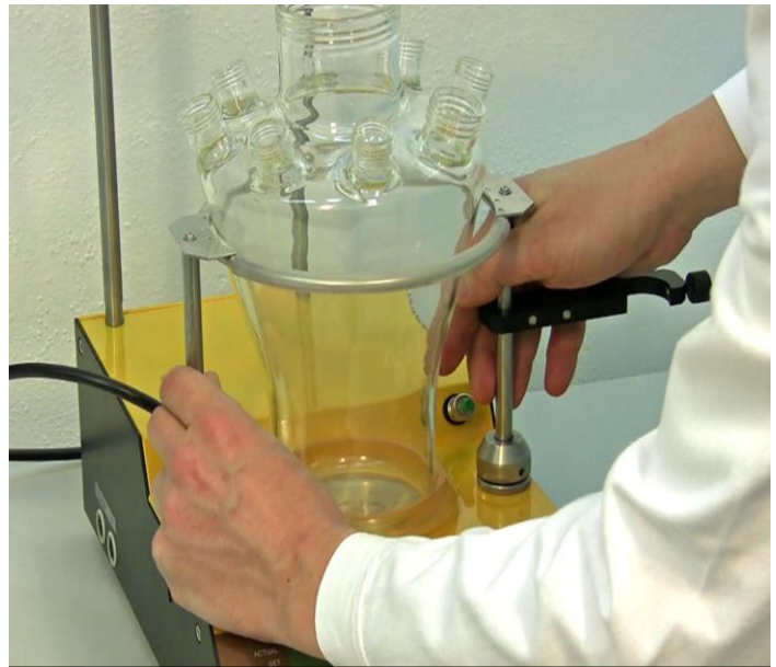
Figure 3.4—10 Adjust the deeply inserted reaction vessel holder around the reaction vessel so that it is supported well. This may be a little stiff, so please be careful.
