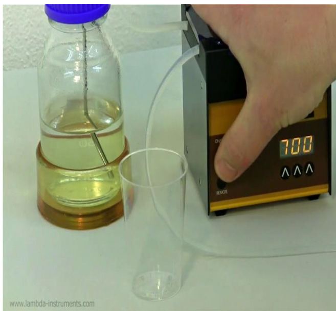
Figure 5.4—8 Switch the pump ON and have the other end of the tubing ready near the measuring beaker.
