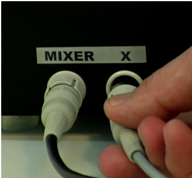
Figure 3.13—3 Connect the weighing module connection cable in the "X" socket beside the "MIXER" on the left side of the MINIFOR base control unit.
