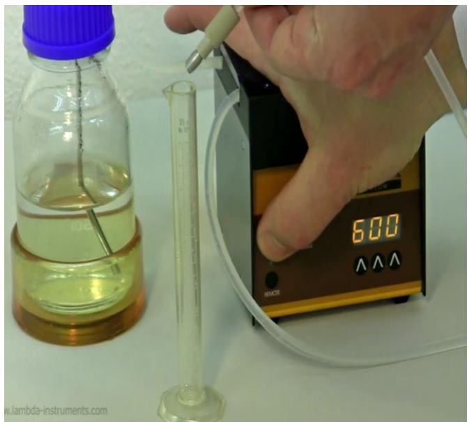
Figure 5.4—2 Turn on the pump and have the other end of the tubing ready near the measuring cylinder. Carefully collect the liquid being pumped in the measuring cylinder for about 60 seconds.
