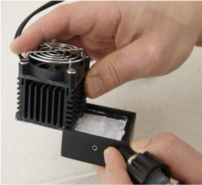
Figure 3.12—6 Detach the Peltier cooling element with control electronics and fan from the condensing finger as shown while preparing for sterilization.
