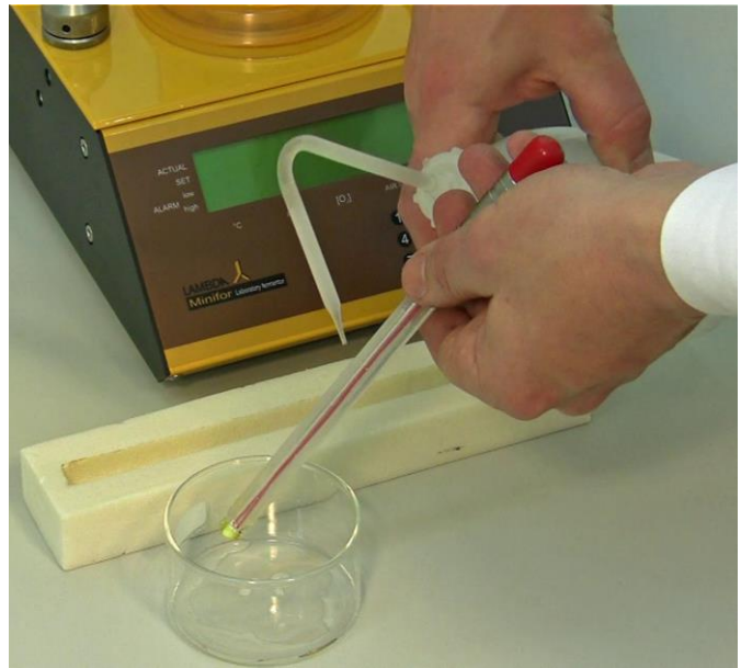
Figure 3.8—6 For smooth insertion of the pH probe on the port, moisten it well with the distilled water.
