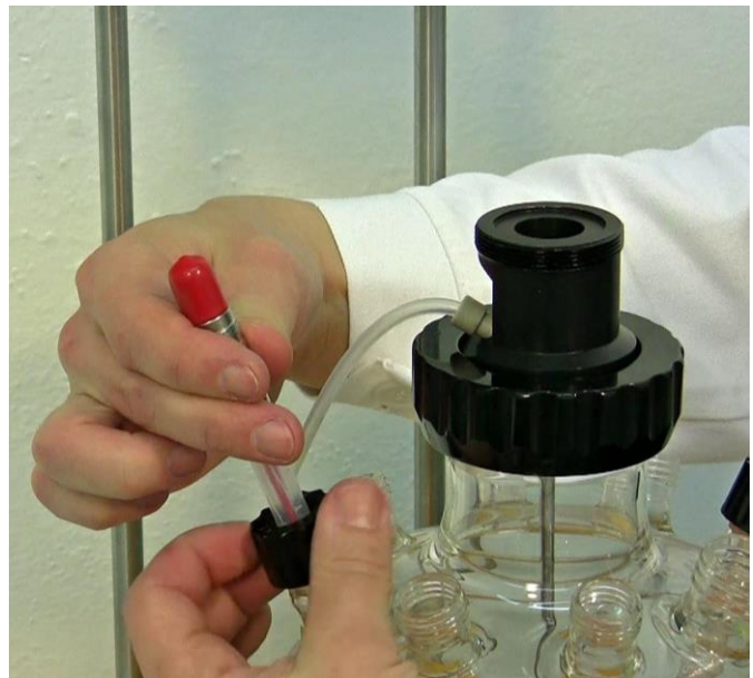
Figure 3.8—8 Tightly secure the black screw cap, after insertion of the pH probe.
