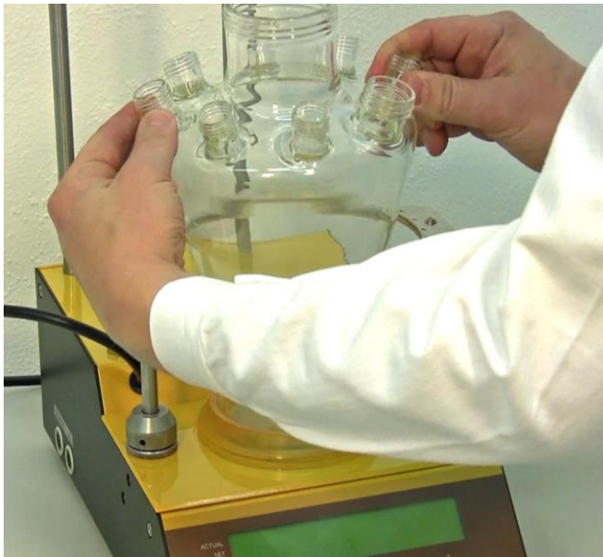
Figure 3.4—9 The port next to the quadruple port is the port usually defined for pO 2 Probe. The port just opposite to pO 2 probe is the port defined for pH probe. These ports for the probes are specially designed (placed nearly on the circumference of the vessel while the other ports are somewhat placed inside) to avoid the interference with the agitation unit.
