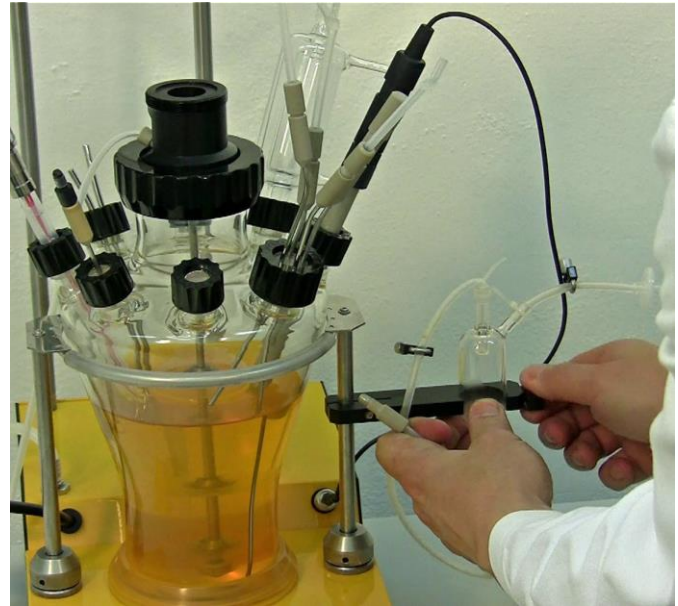
Figure 3.10—24 Place the sterile sampling device on the sterile sampling device holder (Refer 3.4 Setting up of fermentation Vessel) and tighten it with the side-screw.
