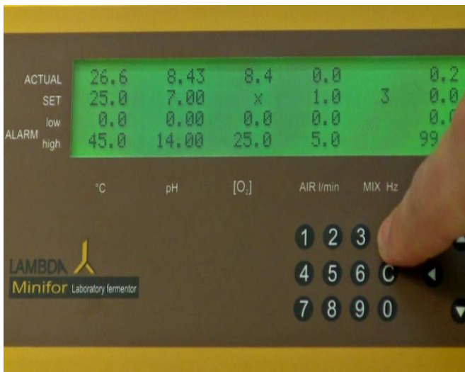
Figure 5.3—14 Press the regulation key "R" to change the calibration mode to standby mode. Since the calibration is just complete, pO 2 probe will be still merged in the O 2 -saturated medium / liquid.
