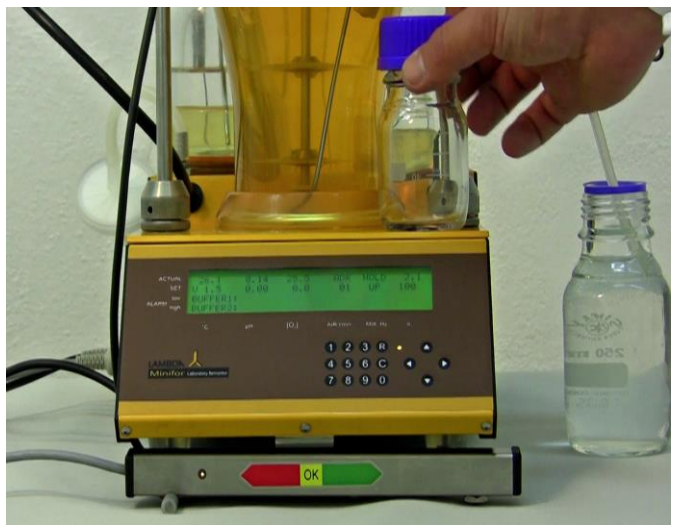
Figure 5.5—6 Place a know weight on the MINIFOR base control unit. For example, place an empty glass bottle.
