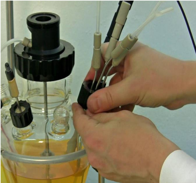
Figure 3.10—23 Insert the quadruple sampling assembly into the port which is larger in diameter and adjacent to pO 2 probe set-up. Fix and tightly secure it with the black screw cap.
