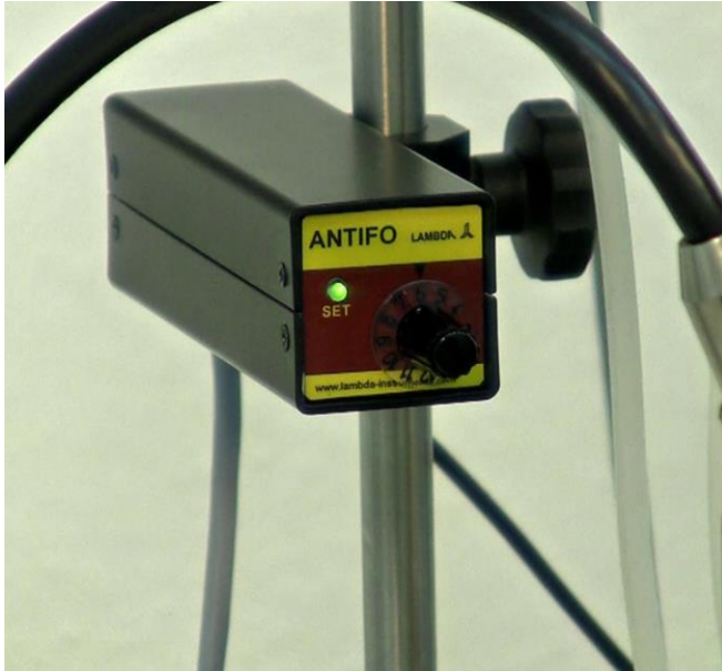
Figure 3.14—1 ANTIFO (foam detector and controller). Place the main body of the ANTIFO on one of the support rods of the MINIFOR laboratory fermenter/bioreactor (e.g. under a pump carrying support). In this way, it will be accessible and occupy minimal space.
