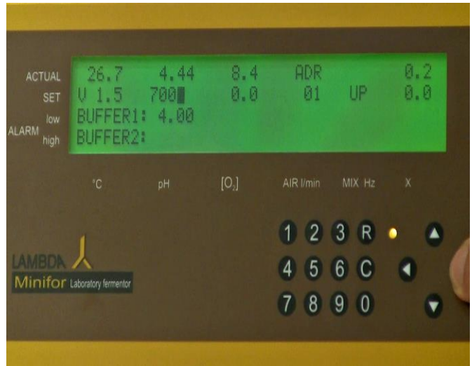
Figure 5.2—10 Start the calibration of the second guaging solution, by entering the next pH value and then press the right arrow key “>” to SET the needed pH value.
