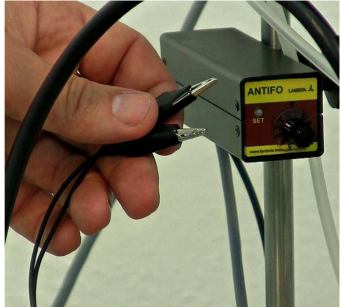
Figure 3.14—2 The two crocodile clips of the ANTIFO need to be connected with the cannulas from the quadruple sampling port for the detection of the foam level in the working vessel.
