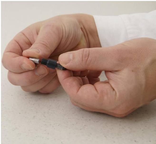
Figure 3.9—1 Insert one end of the double-conical tubing insert to the over pressure security valve.
