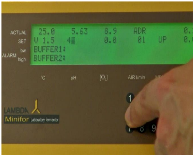
Figure 4.1—7 The number key is used to change the value of the blinking cursor.
