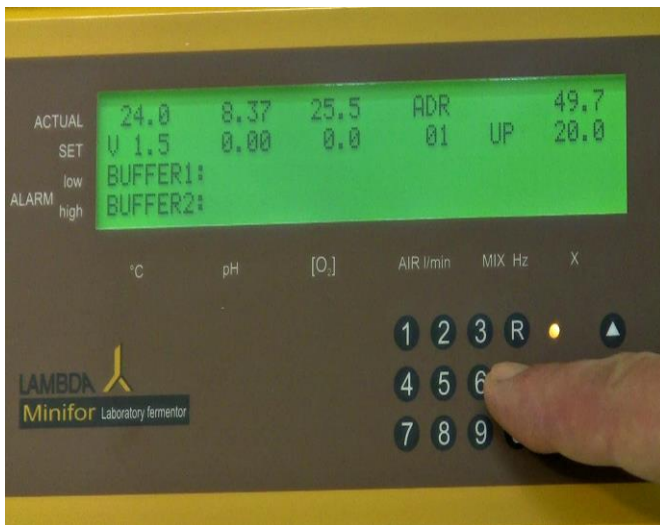
Figure 5.5—14 To change the pump regulation, press the calibration key "C" to change the standby mode to calibration mode.
