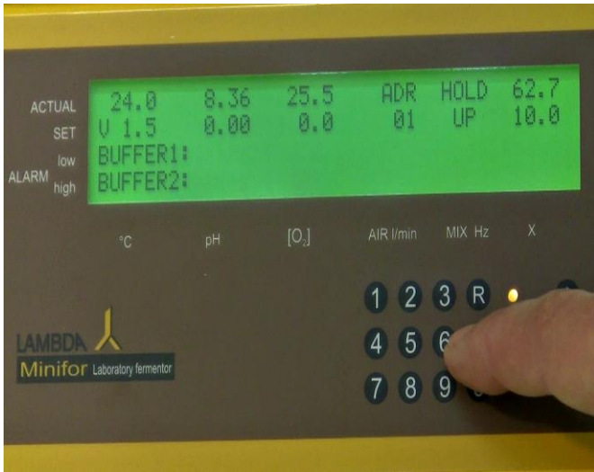
Figure 5.5—7 Observe the actual value of the measured weight. When the reading becomes stable, wait until the message “HOLD” appears. And then press the calibration key “C” to calibrate the initial value.
