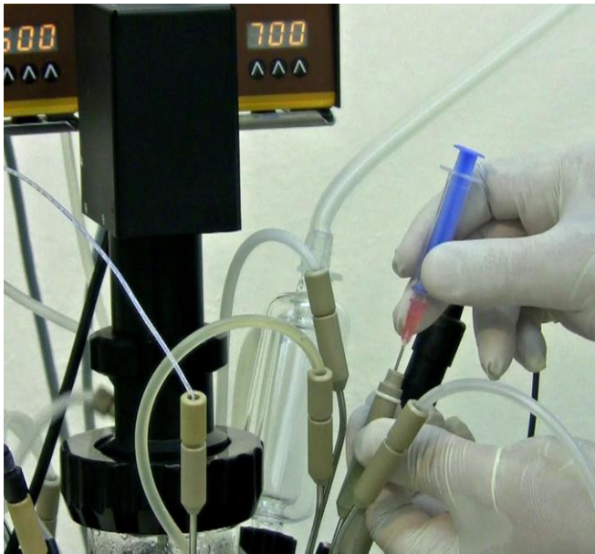
Figure 8.2—5 Remove the syringe along with its needle from the septum adaptor body.
