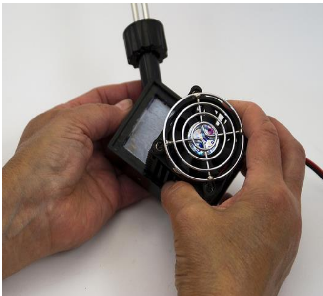
Figure 3.11—7 Detach the motor and fan unit from the cooling pipe as shown while preparing for sterilization.
