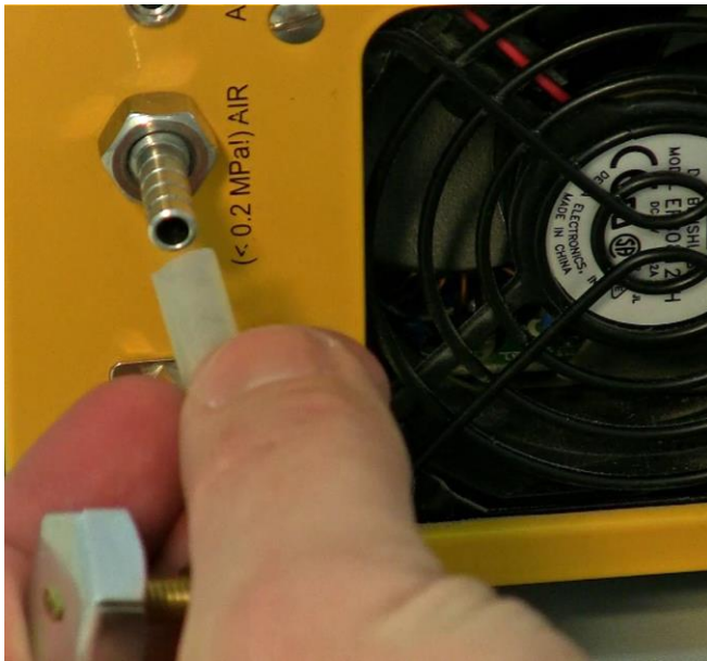
Figure 3.15—21 Connect the air tubing connector, that provides pressurized gas < 0.2 MPa, on the rear of the MINIFOR base control unit. The connection socket will be labelled as ( < 0.2 MPa) AIR to avoid confusion.
