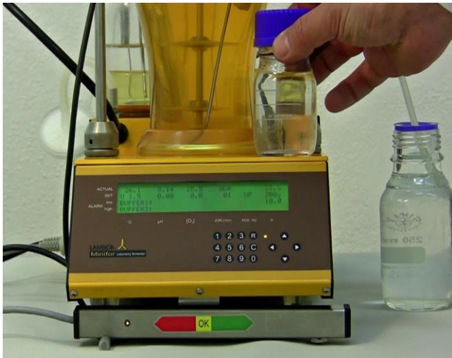
Figure 5.5—9 Then place a known weight or add a certain known volume of liquid to the glass bottle. Say 100 g or ml.
