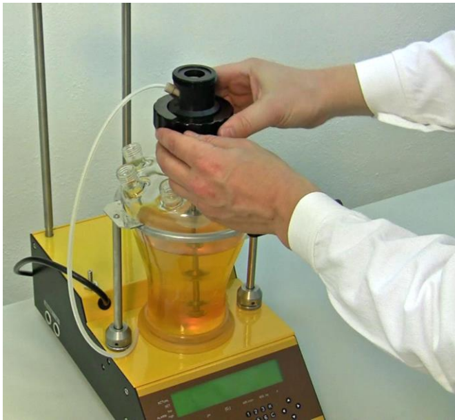
Figure 3.6—1 Take the free end of the air-input tubing (double seal connector tubing attached with mobile cock) from the head of agitation unit as shown.
