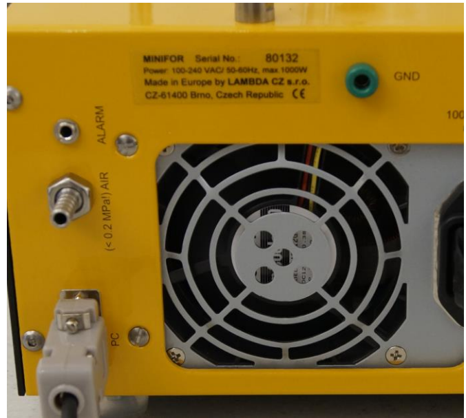
Figure 3.15—41 The alarm connector cable plug has to be connected into the alarm socket at the rear of the base control unit. Other end of the cable can be connected to the desired devices.
