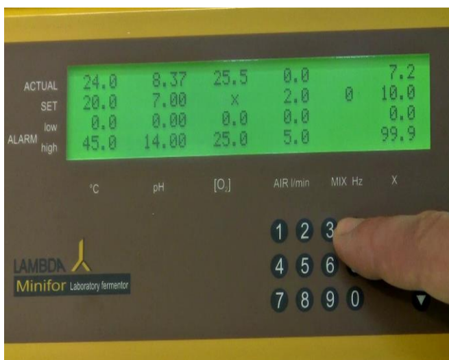
Figure 5.5—19 Press the regulation key "R" to exit the calibration mode.
