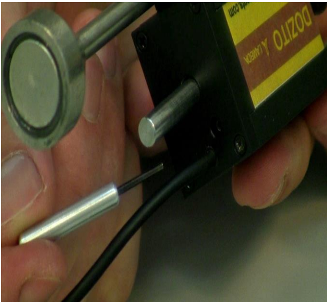
Figure 5.6—5 Use the key given with the ANTIFO and DOZITO kit for setting up the volume of the anti-foam agent added.
