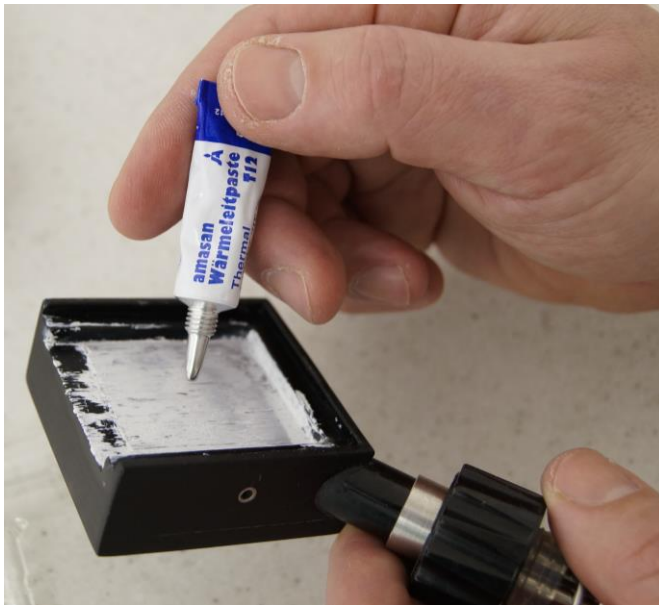
Figure 3.12—8 Apply the heat-conductive paste on the white surface of the Peltier cooling element with control electronics and fan, before attaching the condensing finger with the unit. Spread out the heat-conductive paste on the surface evenly and thinly ensuring that there are no trapped air bubbles.
