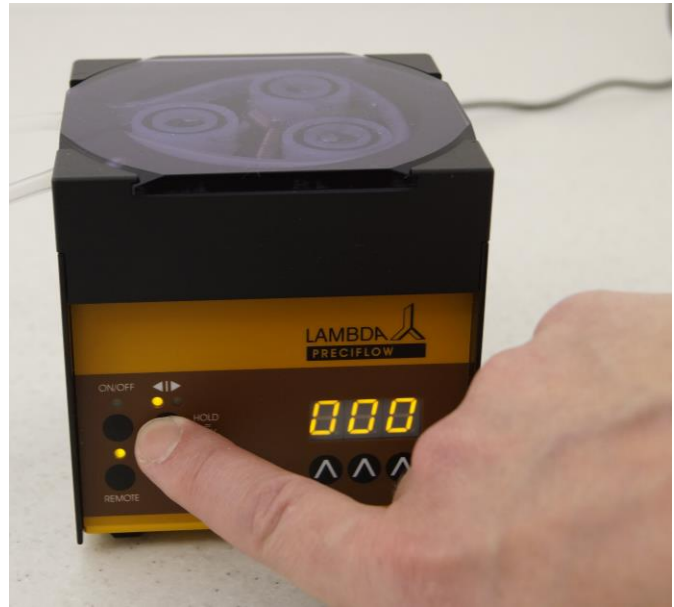
Figure 3.13—9 Press the remote button on the connected 'X'-channel Peristaltic pump.
