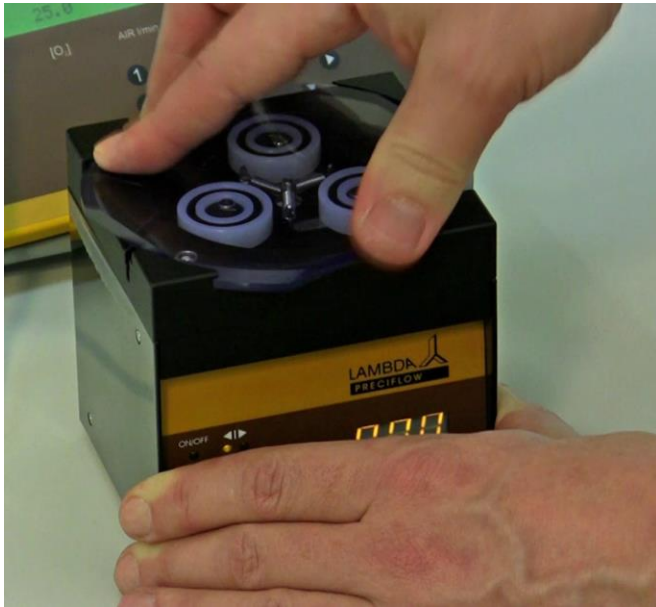
Figure 3.16—1 For the installation of tubing into the Peristaltic pump, twist the transparent PVC head cover either clockwise or anti-clockwise to remove.
