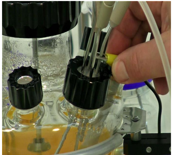
Figure 7.1—4 Remove the grounding cable from the reaction vessel cannula.
