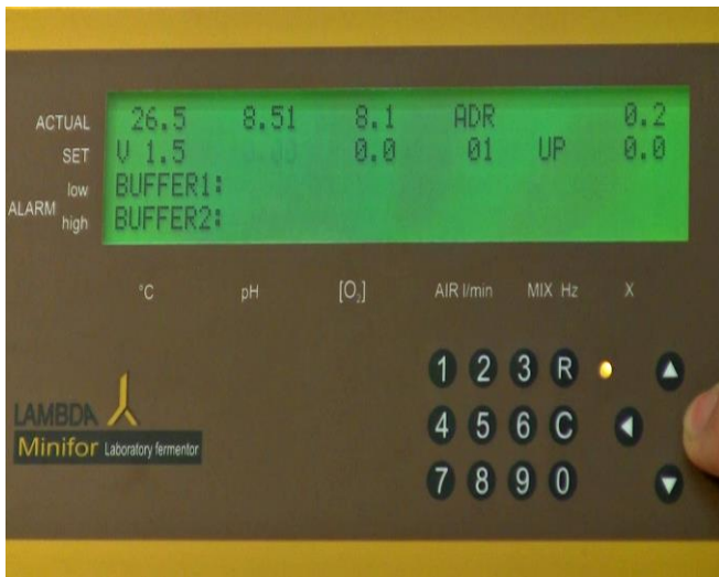
Figure 5.5—3 Once the cursor is activated, use the right navigation key (>) to choose the parameter “X”.
