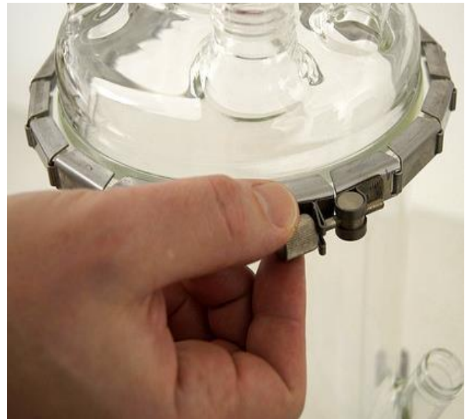
Figure 3.4—28 Fix them together with the segmented vessel closing belt. The mixture will cure either during staying at room temperature in several hours or within minutes in the autoclave during sterilization.
