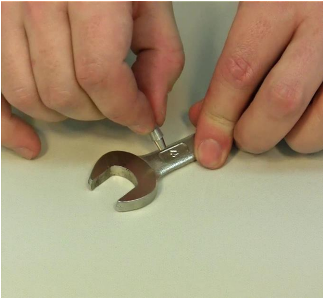
Figure 3.10—9 Take a spanner and the double seal conical insert with the tubing. Press the conical insert with the tubing against the spanner to make it inserted totally into the tubing.
