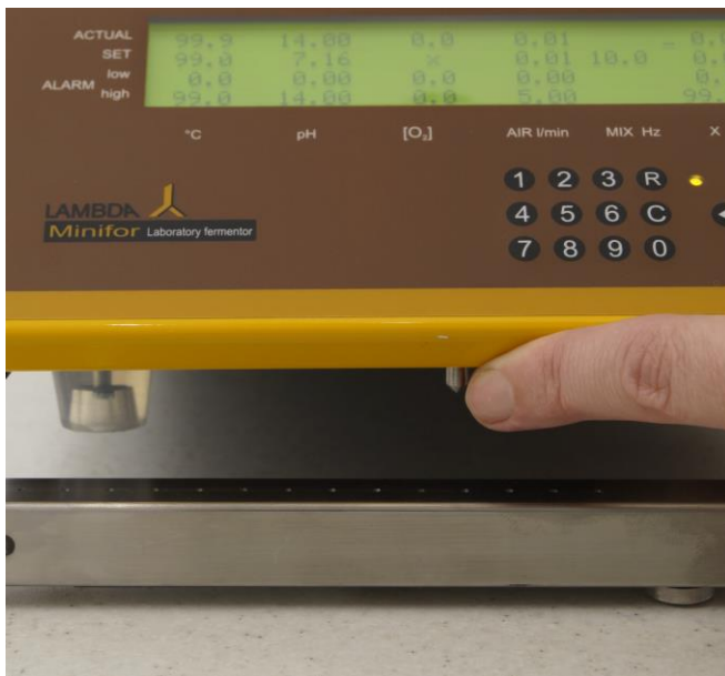
Figure 3.13—1 The steel hard tip can be found under the front part of the MINIFOR unit (miniature scale module). Place the weighing module under the front part of the MINIFOR.
