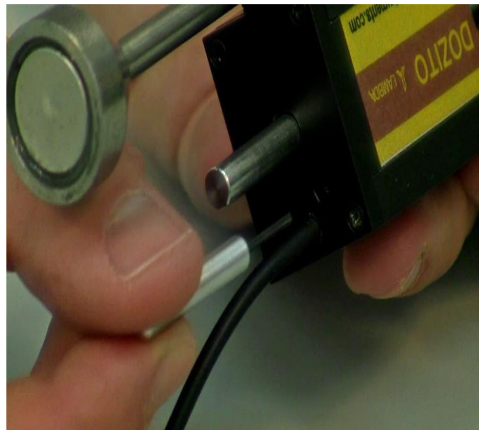
Figure 5.6—8 screwing out = counter-clockwise rotation = increase of the delivered antifoam volume / step
