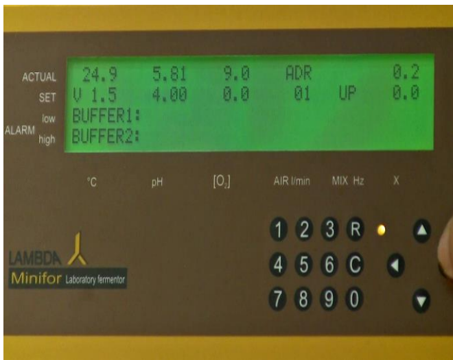
Figure 5.2—5 Press the right arrow ">" to SET the blinking value. Please note that after pressing the right arrow, the value 400 changes to 4.00.
