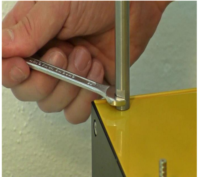
Figure 3.3—2 Further fix the inserted support rod tightly with the supplied spanner.
