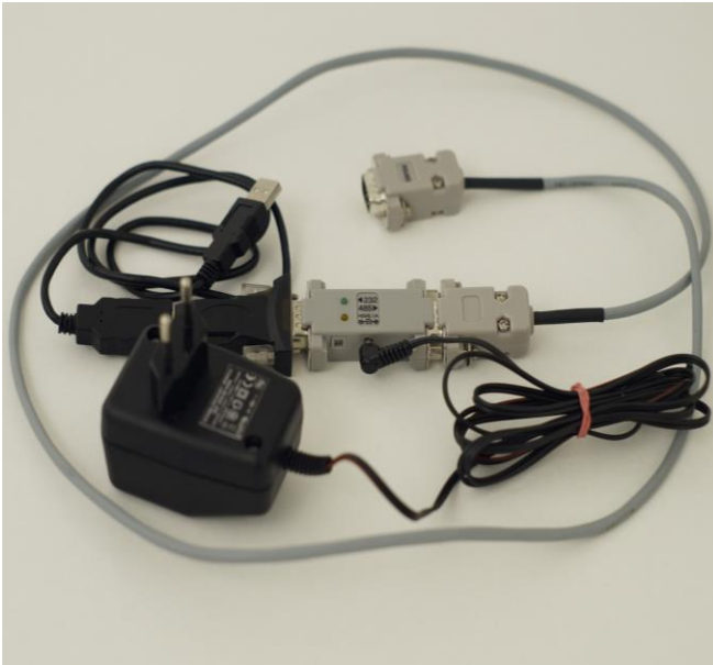
Figure 3.15—38 PC connection kit with RS-485 to RS-232 converter and USB connection.
