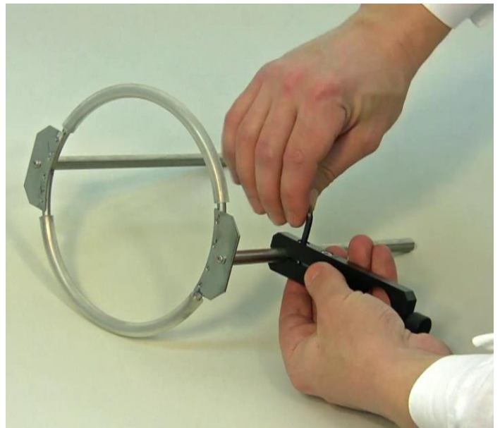
Figure 3.4—4 After inserting the sterile sampling device holder and positioning it, fix the corresponding screws as shown with the given key to make it hold firmly.
