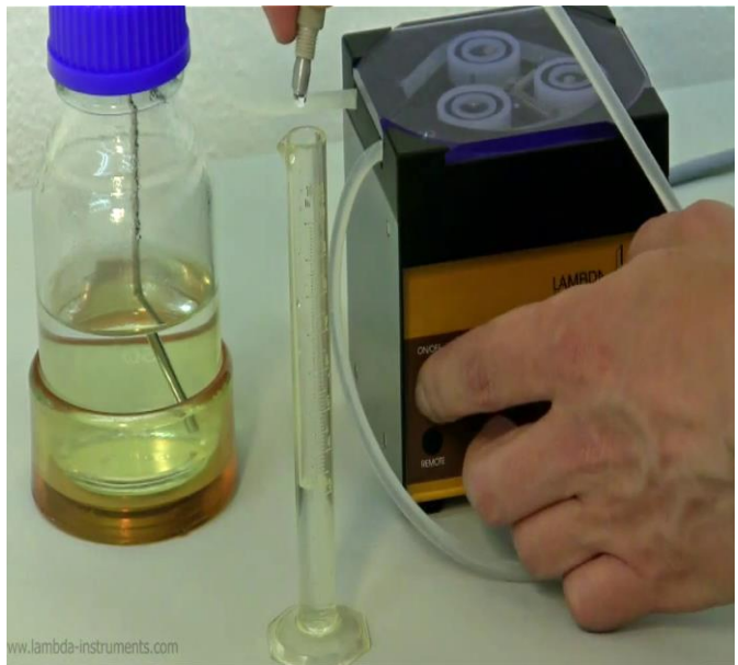
Figure 5.4—4 Exactly after 60 seconds, switch off the pump.
