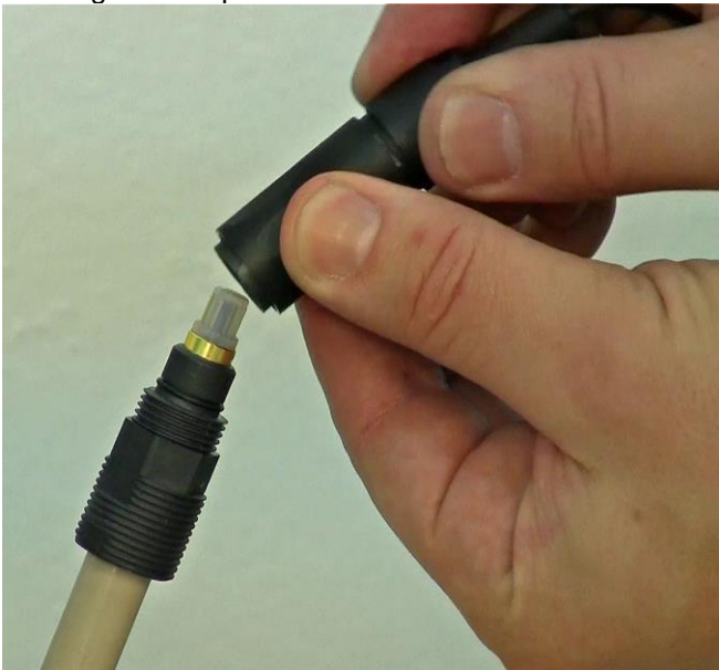
Figure 3.7—11 pO 2 (DO) probe connector have to be connected between the pO 2 probe and the pO 2 (DO) probe socket in the base control unit. Adjust the sleeve of the pO 2 (DO) probe connector by pushing it up as shown.
