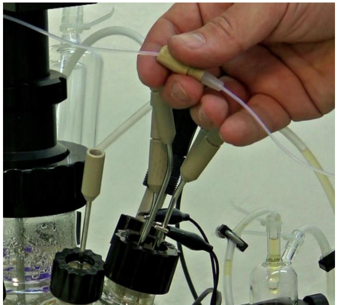
Figure 3.14—26 The PTFE antifoam line has to be connected with the shortest cannula that will facilitate the addition of antifoam above the liquid level.
