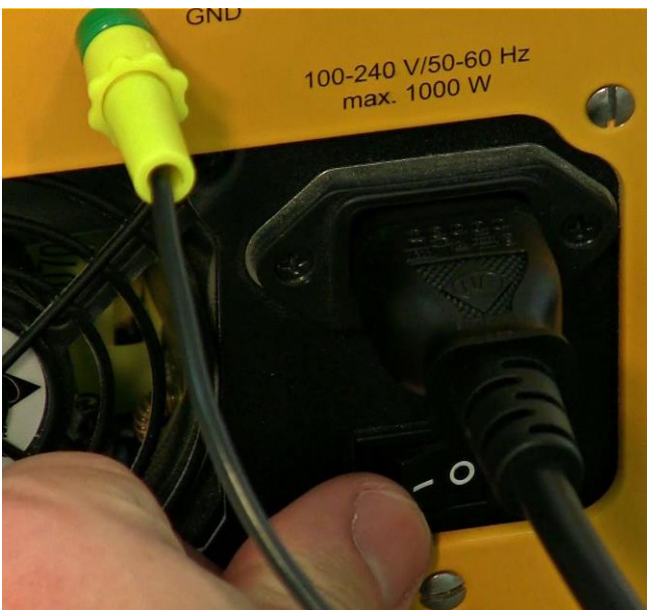
Figure 3.15—44 Once the connections and installations are done, switch on the MINIFOR using the power switch present below the power input. (Power Switch: I = On; O = Off)
