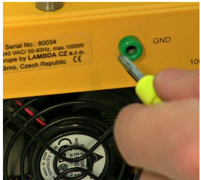
Figure 3.15—35 Connect the black cable with green connector to "GND" at the rear of the MINIFOR base unit for grounding (or earthing).
