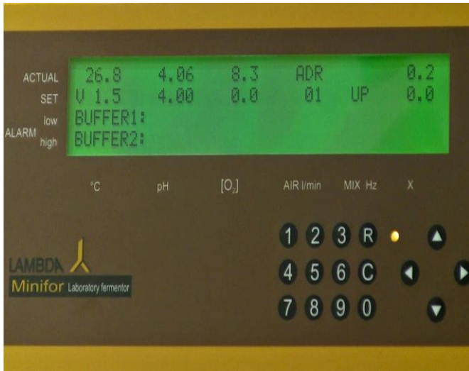
Figure 5.2—7 The pH of the buffer will be displayed on the ACTUAL value of the pH (above the SET value). Wait until the ACTUAL value of the pH gets stable.
