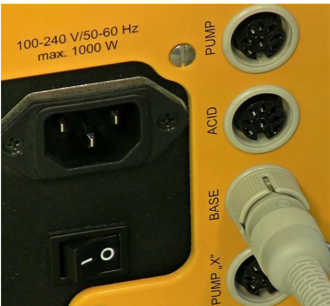
Figure 3.16—16 Connect the base Peristaltic pump cable into the 'BASE' socket on the MINIFOR base control unit.
