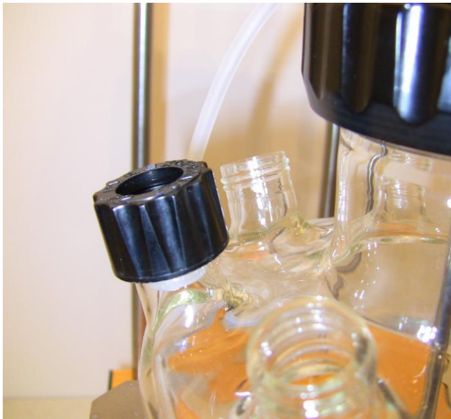
Figure 3.8—5 Place the black screw cap loosely on the white open stopper and washer.
