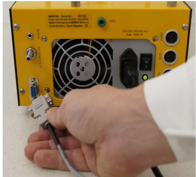
Figure 3.15—39 Connect the PC connection cable to the DB 9 connector at the rear of the base control unit.
