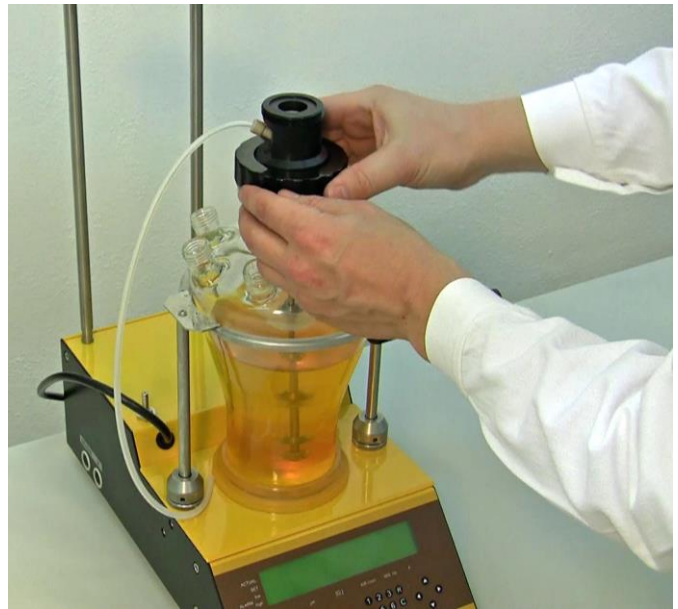
Figure 3.5—26 Ensure that the large central screw cap for head fixing is securely tightened to the rim of the reaction vessel. See that the mobile PEEK cock tubing for air input is positioned as in the figure.
