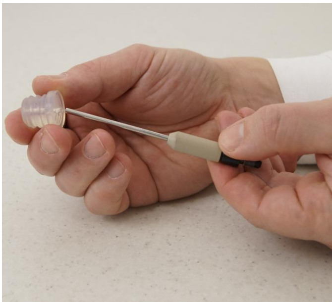
Figure 3.9—3 Insert the assembled over pressure limiting security valve to the rubber stopper.
