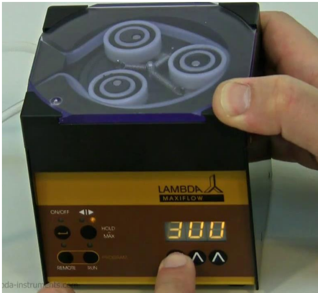
Figure 3.16—10 The \wedge \wedge \wedge buttons can be used to set the desired flow rate.
