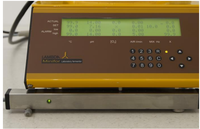
Figure 3.13—6 If the vessel weight is too low, an underscore sign “_” will appear along with the measured (actual) weight value [Refer Actual value of the parameter “X”] and a green LED light will be displayed in the weighing module.
