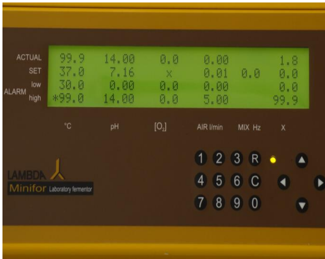
Figure 4.3—6 Alarm high is activated. * sign can be seen with the alarm high value.
