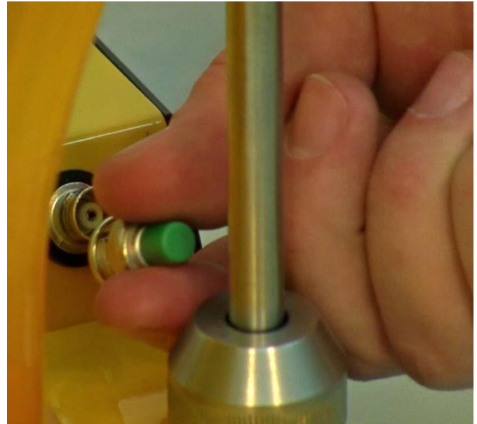
Figure 3.7—14 Remove the protection cap by pressing and unlock by rotating from the pO 2 (DO) probe socket on the base control unit.
