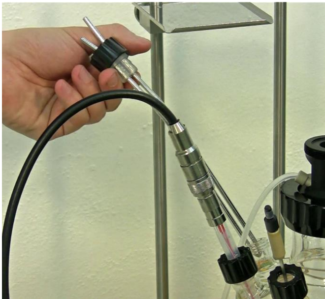
Figure 3.11—3 Place the cooling loop in the desired neck at the back of the vessel to leave it undisturbed.
