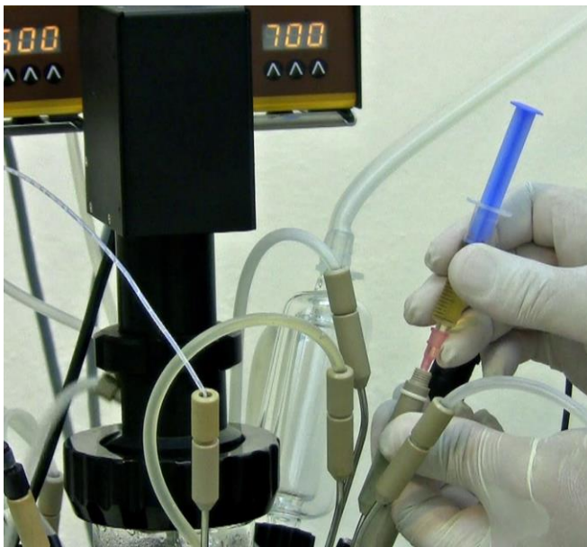
Figure 8.2—3 Insert syringe loaded with the inoculant / inoculum along with the syringe needle to the septum adaptor body.
