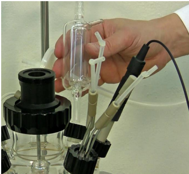
Figure 3.12—2 Glass outgas condenser and gas outlet filter need to be sterilized together with the MINIFOR vessel.
