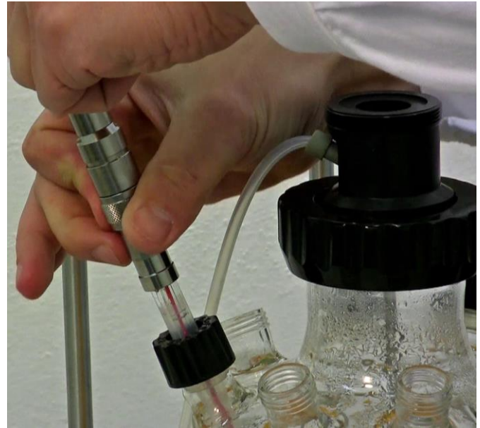
Figure 3.15—8 After locking the pH probe and connector cable; tighten the connection by screwing the threaded lock on the connector cable by rotating as shown.
