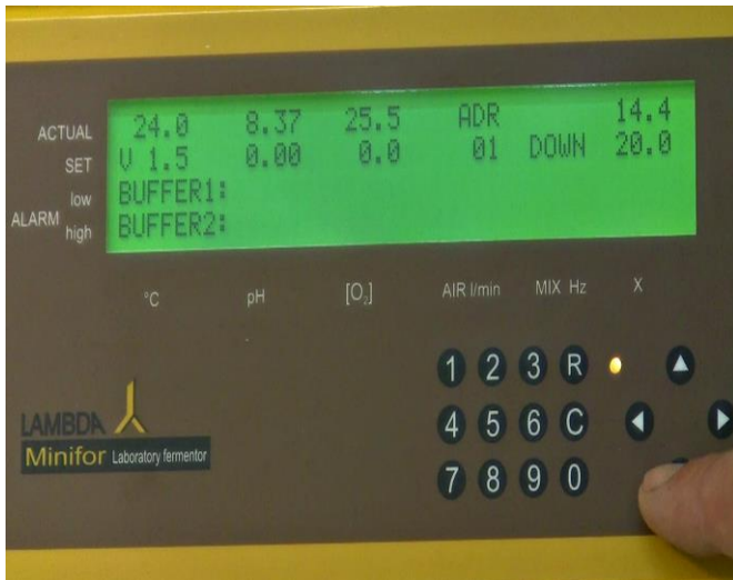
Figure 5.5—16 Use the down navigation key to change to DOWN option.
