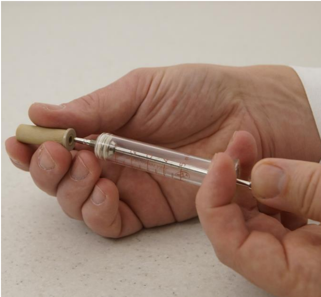
Figure 3.14—7 Push the plunger completely along the barrel of the syringe to mechanically fix the metal outlet tip. Insert the PEEK adapter body on the threaded syringe tip and tighten it securely by screwing.
