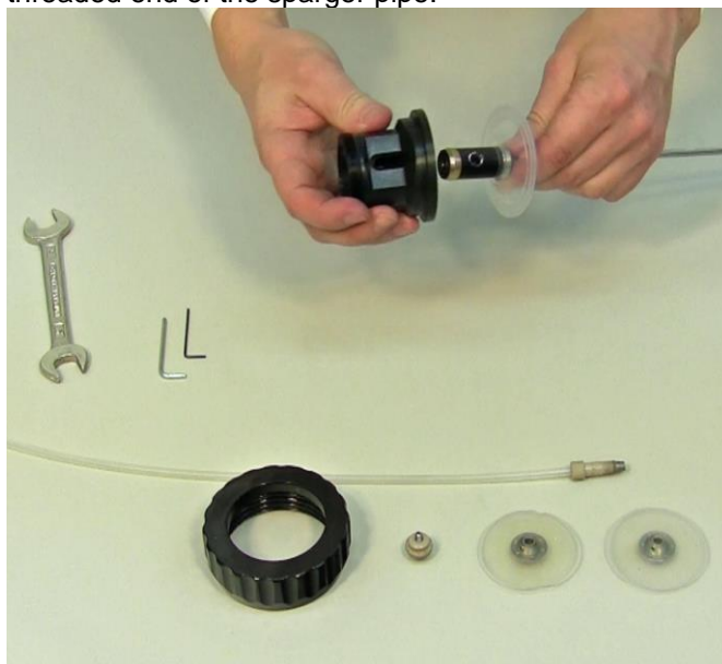
Figure 3.5—16 Place the head of the agitation unit above the prepared mobile cock with silicone sterility membrane in the sparger pipe.
