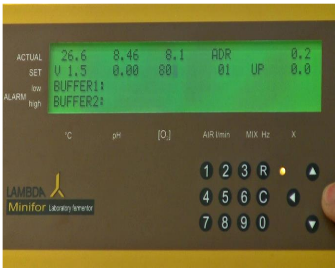
Figure 5.3—5 Enter the value from the table in the SET [O 2 ] and then press the right arrow key (>). (e.g.: 80)
