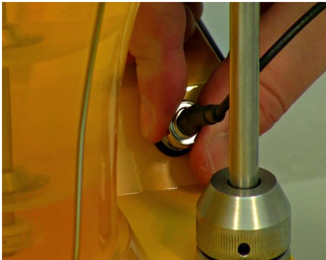
Figure 5.3—8 For the Zero point calibration, disconnect the pO 2 (DO) probe.
