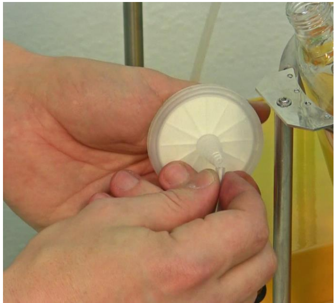
Figure 3.6—2 Connect the air-input tubing from the agitation unit to one end of the air-input filter.
