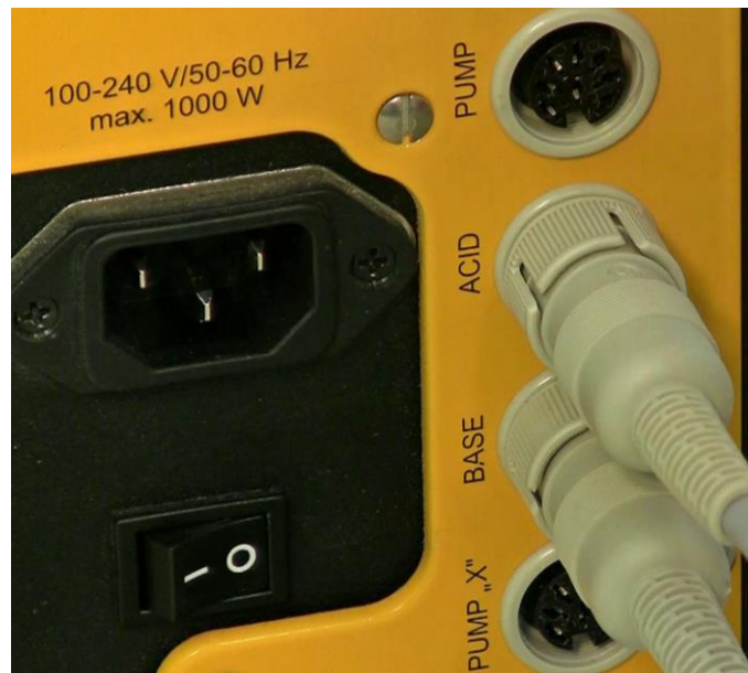
Figure 3.16—17 Connect the acid Peristaltic pump remote cable into the 'ACID' socket on the MINIFOR base control unit.
