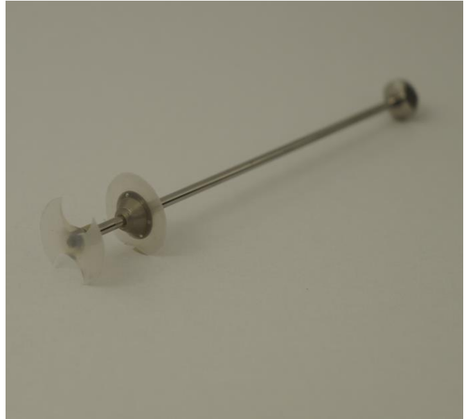
Figure 3.5—28 Butterfly shaped stirrer disc mounted on the sparger pipe instead of the self cleaning microsparger for 0.3L vessel.
