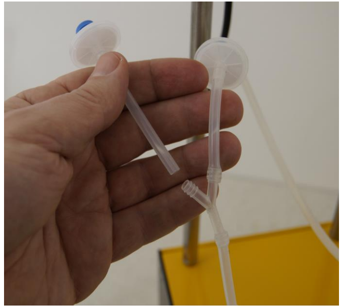
Figure 3.6—12 Insert another tubing with the filter to the Y-piece for surface sparging.
