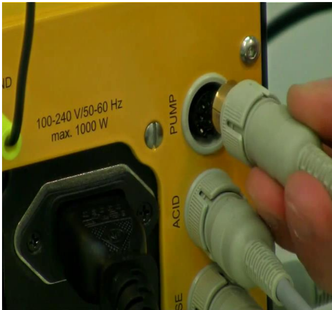
Figure 3.15—9 Peltier cooling finger can be directly connected on the “PUMP” socket present at the rear of the MINIFOR base control unit.
