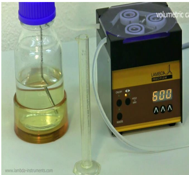
Figure 5.4—1 Connect the tubing to liquid in the bottle and set the desired speed (e.g. 600). Keep the measuring cylinder ready.
