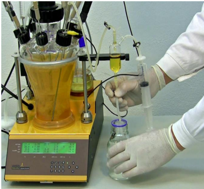
Figure 8.2—5 Remove the 70% Ethanol beaker / bottle into which the outlet tubing is dipped.
