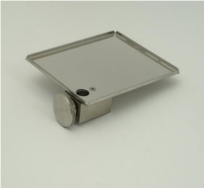
Figure 3.3—5 The adjustable support plate that needs to be inserted on the support rods. (N.B: In case, the LAMBDA Peristaltic pumps are used, for example: controlled addition of acid and base to maintain the pH).
