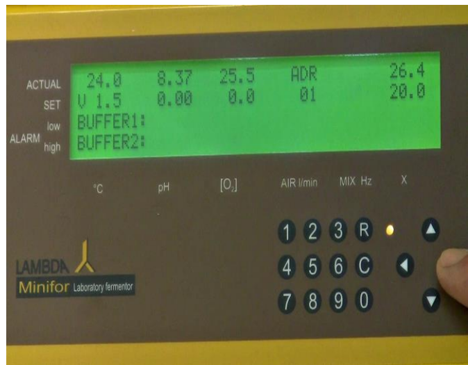
Figure 5.5—15 Press the right arrow navigation key (>) to select the SET value "UP" in the column before the parameter "X".
