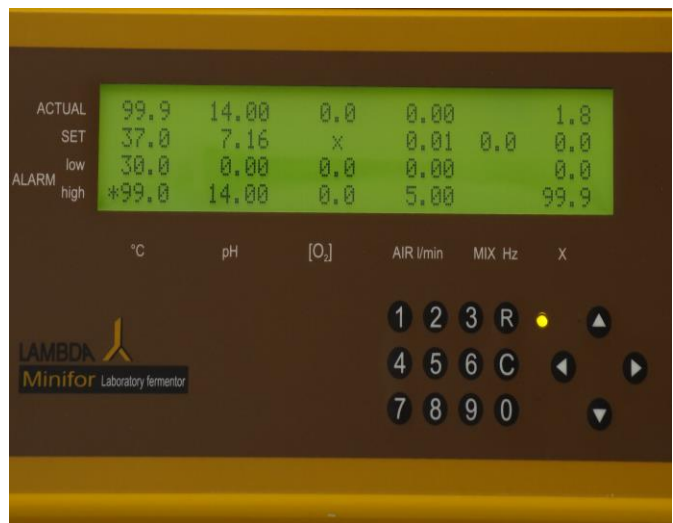
Figure 4.3—4 Move the cursor on the field of temperature maximum (ALARM HIGH). Enter the desired value. If the temperature exceeds this value, an alarm is activated and the exceeded value is highlighted on the display.
