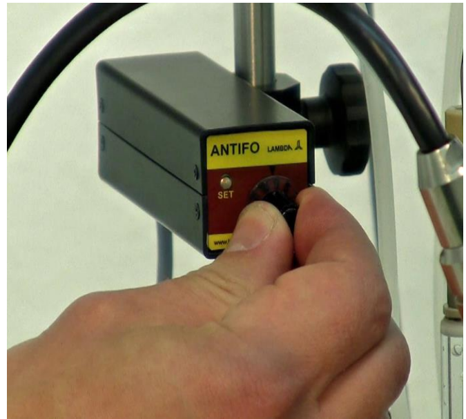
Figure 5.6—2 Rotate the ANTIFO knob clockwise gently to find a point where the green LED turns to yellow as shown.
