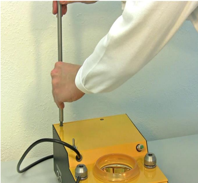
Figure 3.3—1 As a first step, insert the support rods in the present basic control unit as shown. Rotate it clockwise for fixing.
