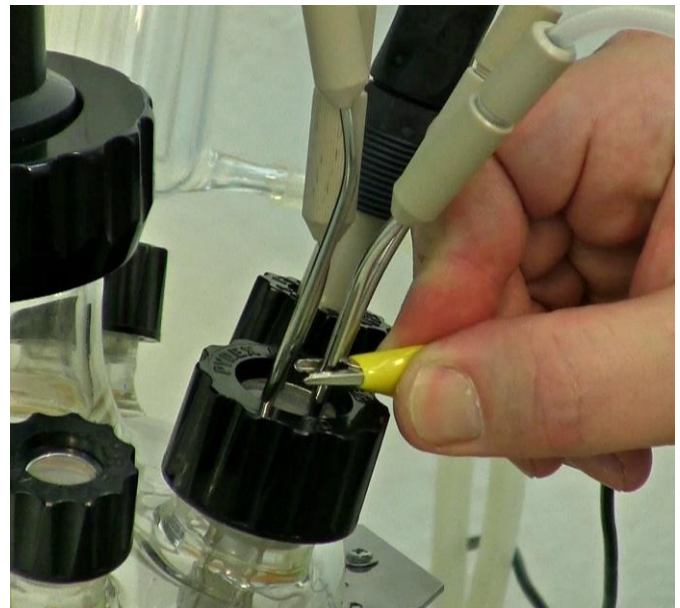
Figure 3.15—37 Clamp the other side of the grounding cable with yellow crocodile clamp to the longest cannula of the quadruple sampling port.
