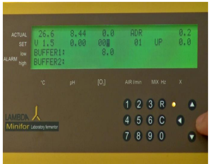
Figure 5.3—11 Enter the SET [O 2 ] value 00 using the number keys and press the right arrow ket to save the value. The value will be displayed as 0.0 in the SET value.
