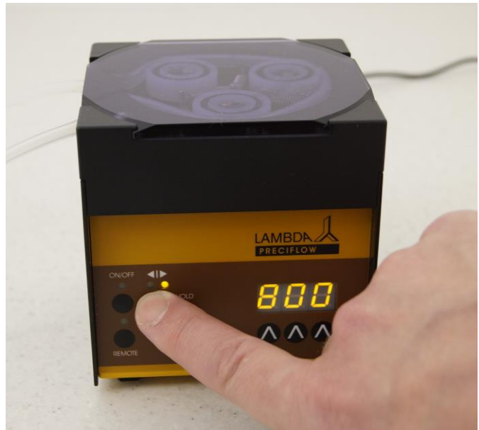
Figure 3.16—13 LED illumination in the direction |▶ represents the anticlockwise rotation.
