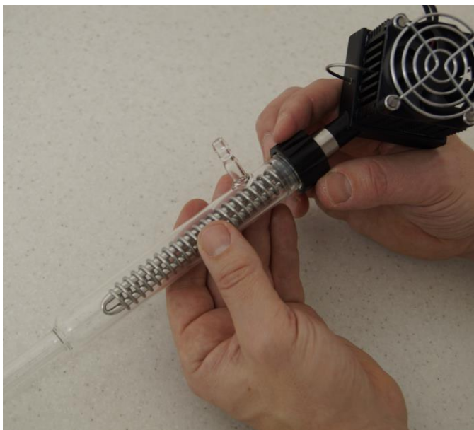
Figure 3.12—12 Insert the outgas condenser cylinder with the tubing connection over the condensing finger and tighten it securely by the black screw cap.
