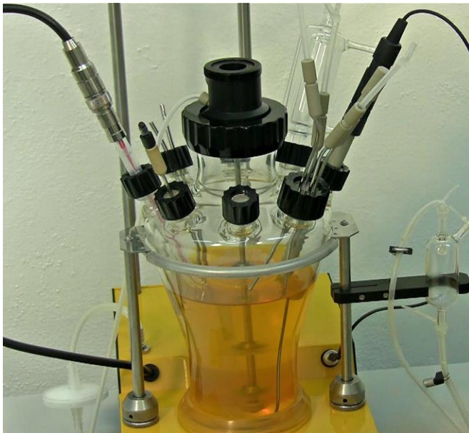
Figure 7.1—1 Fill 3/4th of the reaction vessel with buffer or medium.
