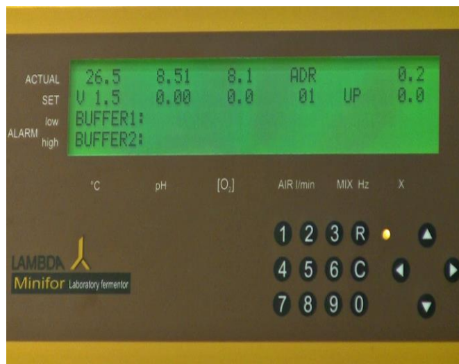
Figure 4.2—3 Calibration mode - Key "C" starts the calibration of pH, pO 2 , parameter X or the setting of the address for PC control (depending on the choice with the cursor). The LED is yellow and the regulation is off. (Only the agitation is activated to allow precise calibration of pO 2 probe).
