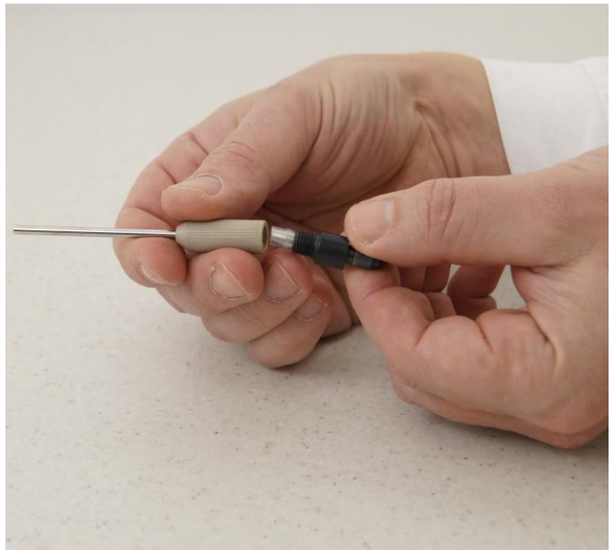
Figure 3.9—2 Insert the other end with the stainless steel cannula with LAMBDA PEEK connector.
