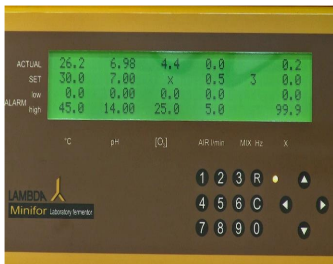
Figure 4.2—1 Standby mode - state of the fermenter after switching on. The display shows the last entered parameters. In this configuration all measurement readings are shown, but the regulation is switched off and the number keys blocked. LED is yellow and all numbers on the display are static.
