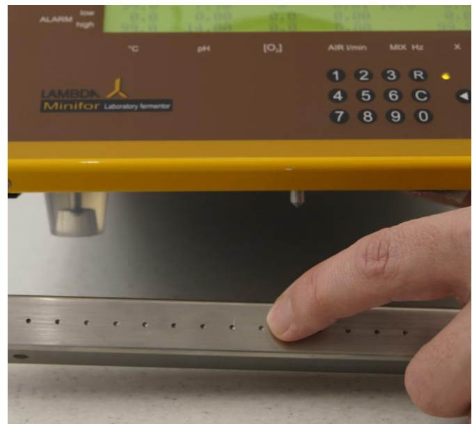
Figure 3.13—2 The steel tip (miniature scale module) under the front of the MINIFOR unit should be placed in these grooves of the weighing module.
