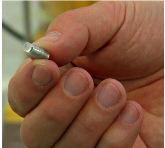
Figure 3.10—12 The tubular septum (which is sealed at one end) should be fitted over the double seal conical insert with the use of, for example, a hard ruler leaving part of the tubular septum free and exposed as shown.
