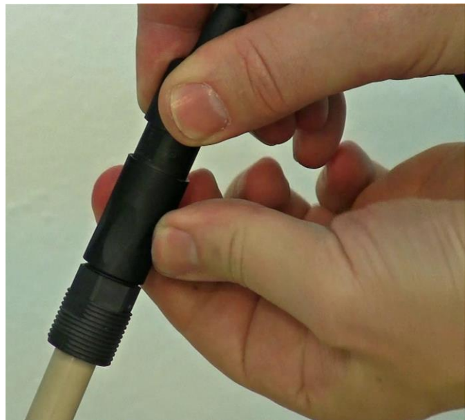
Figure 3.15—18 After fixing the pO 2 (DO) probe and connector exactly in locking position, push down the sleeve of the pO 2 (DO) probe connector and secure it sufficiently with screw fitting.
