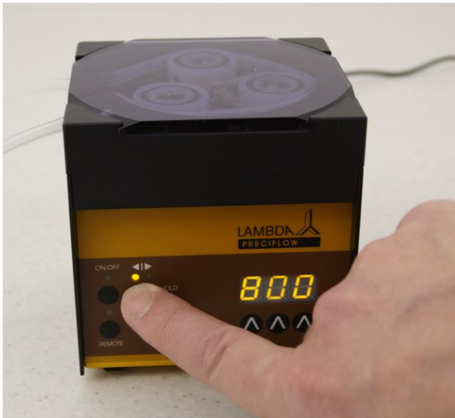
Figure 3.16—12 LED illumination in the direction ◀| represents the clockwise rotation.
