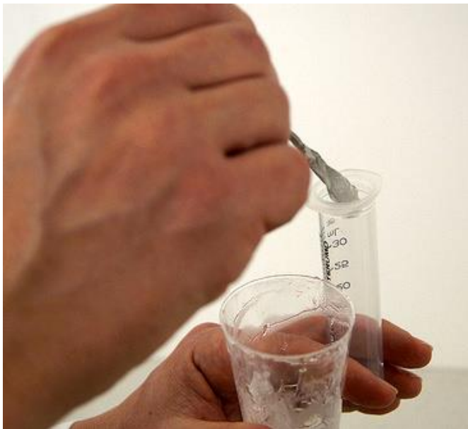
Figure 3.4—23 Transfer the prepared liquid O-ring into a syringe for an easy application of the mixture in the vessel.
