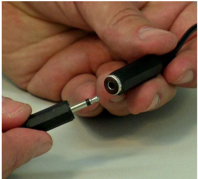
Figure 3.15—32 Plug in the DOZITO's black cable to the floating black cable of ANTIFO, as shown.
