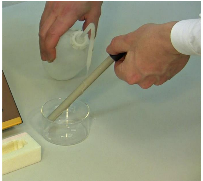
Figure 3.7—8 Moisten the pO 2 (DO) probe with de-ionized water to ease insertion of probe.
