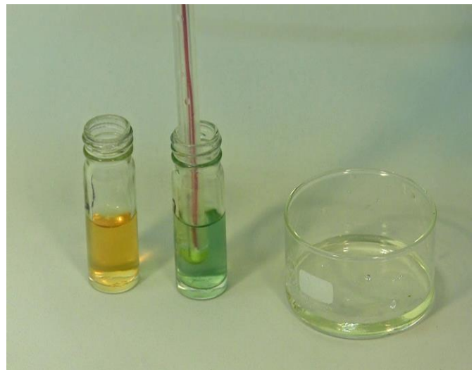
Figure 5.2—12 Dip the pH probe into the pH 7 buffer solution and gently stir it, until the pH value becomes stable.
