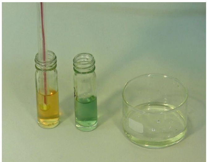
Figure 5.2—22 Now the measurement of pH 4 can be checked by dipping the probe into pH 4 buffer solution.
