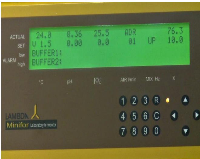
Figure 5.5—5 Entered 100 will appear as 10.0 in the SET display after pressing the right arrow key.
