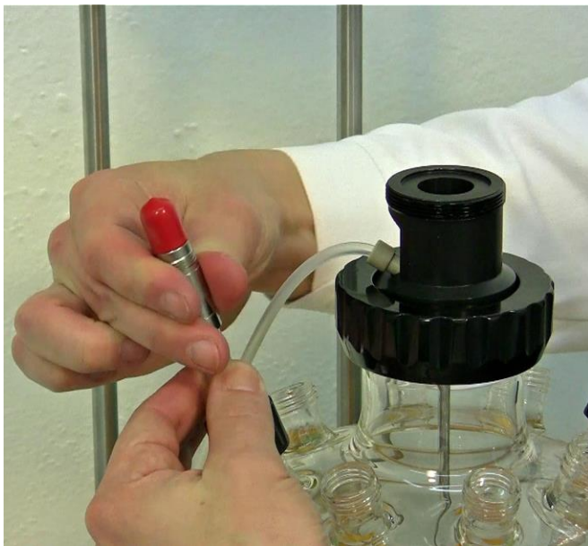
Figure 3.8—7 Carefully insert the pH probe on the pre-prepared port with the stopper, washer and black screw cap.
