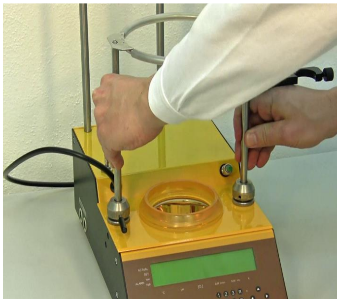
Figure 3.4—6 The vessel reaction holder with the sterile sampling device holder needs to be fixed on the MINIFOR base control unit. Place the reaction vessel holder in the 2 desired slots on either side of the sun-like heating element.
