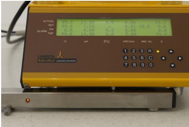
Figure 3.13—5 If the weight of the filled vessel exceeds the measurement range, a roof sign “^” will appear in the measured (actual) weight value [Refer Actual value of the parameter “X” in the display] and a red LED light will be displayed in the weighing module.
