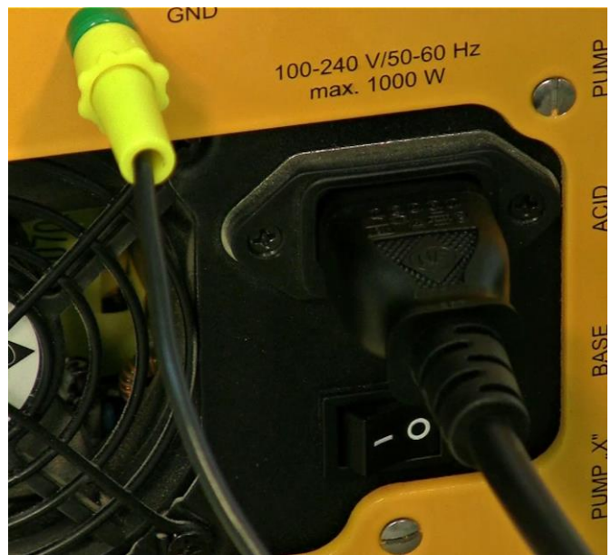
Figure 3.15—43 Connect the Power cord to the power inlet (100-240 V/ 50-60 Hz) at the rear of the MINIFOR base control unit.
