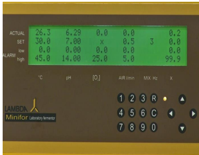
Figure 5.3—17 The 'ACTUAL' reading should show '0' after sometime.
