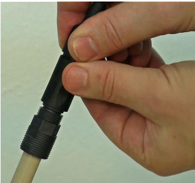
Figure 3.15—17 Place and adjust the pO 2 (DO) probe connector by rotating to find the position for exact locking of grooves with the pO 2 (DO) probe.
