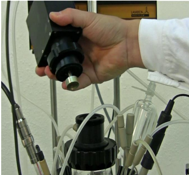
Figure 7.1—5 Remove the agitator from the agitation unit. Carefully tilt the agitator back and forth for easy removal.
