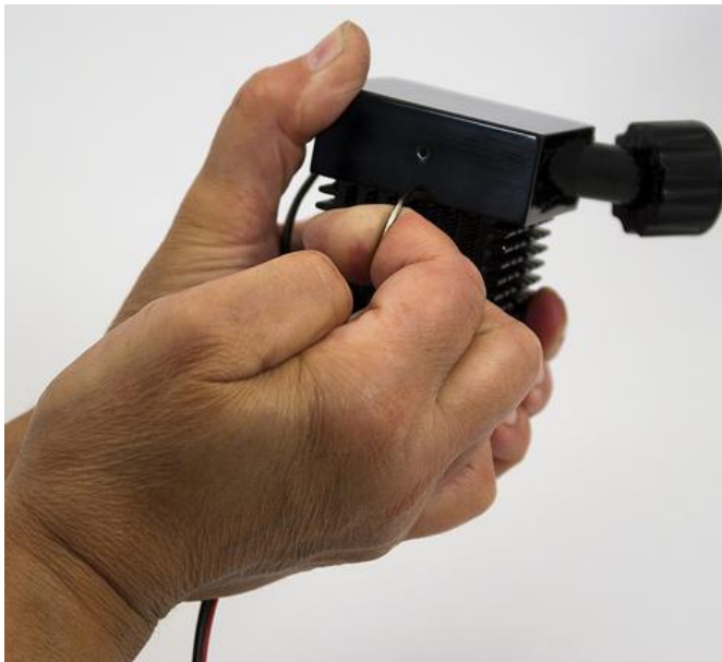
Figure 3.11—13 Locking clamp has to be pulled firmly through the Peltier cooling element with control electronics and fan to make the Peltier cooling finger intact.
