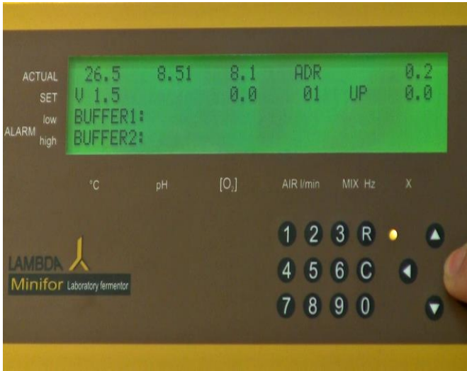
Figure 5.3—3 Move the cursor to the [O 2 ] value using the right navigation key (>).
