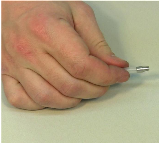
Figure 3.5—8 The resulting double-seal conical insert with the tubing should be like in figure i.e. half the portion of the conical insert can be found inside the tubing.
