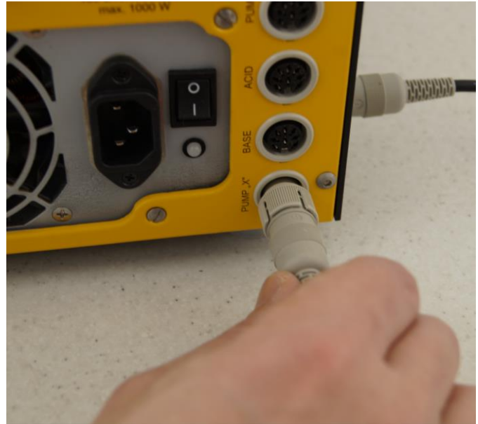
Figure 3.15—26 Connect the corresponding pump (for the addition or removal of medium) to the "PUMP X" socket on the rear of fermenter-bioreactor MINIFOR.
