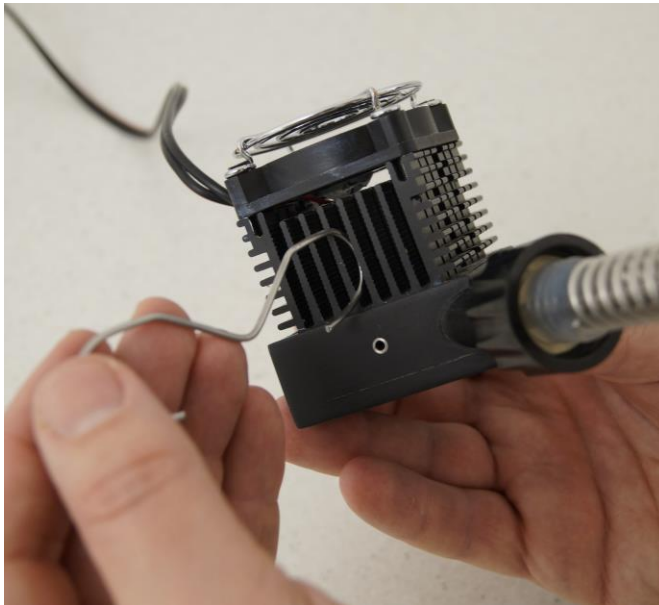
Figure 3.12—10 The attached peltier cell with the condensing finger should be made kept together with the help of the locking clamp.
