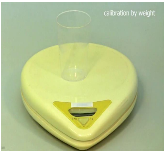
Figure 5.4—6 Measure the weight of the empty beaker using a sensitive weighing scale. For the exact measurement of the liquid collected, tare the weighing scale with the measuring beaker (Example: 0.000 g).
