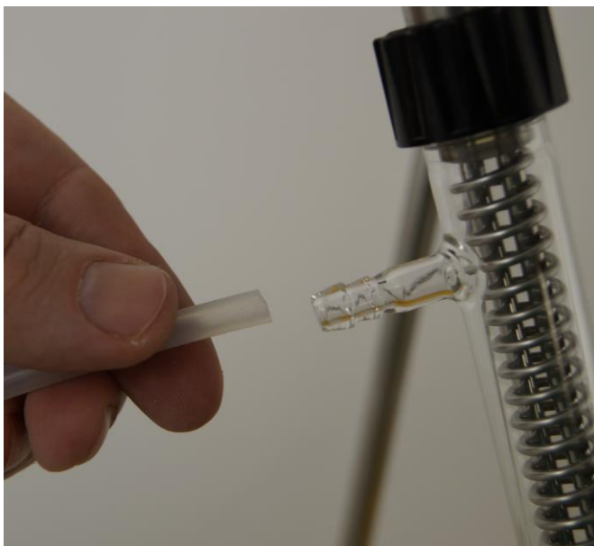
Figure 3.12—14 Connect a tubing to the outgas condenser cylinder and lead the tubing to a glass vessel or flask.
