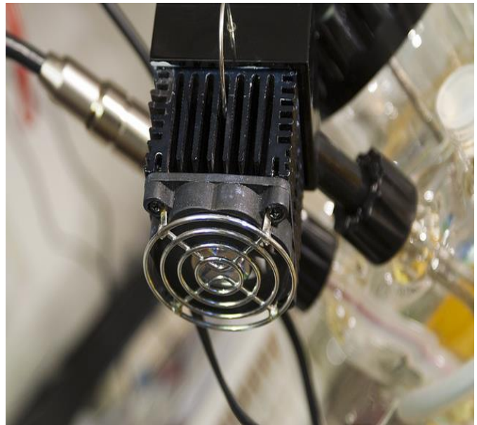
Figure 3.11—14 Peltier cooling finger can be placed in the same place as the cooling loop placed (Refer 3.11.1 Cooling Loop). Secure it tightly with care using the black screw cap, since the head of the Peltier cooling may be slightly heavy while fastening the screw cap.
