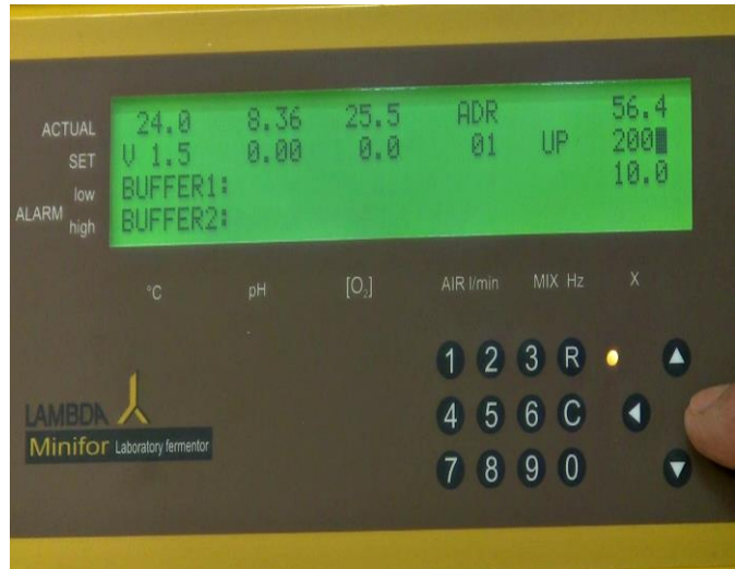
Figure 5.5—10 Enter the final value to be detected and controlled by the scale module. For example: enter 200 and press the right arrow key (>) to save the value.
