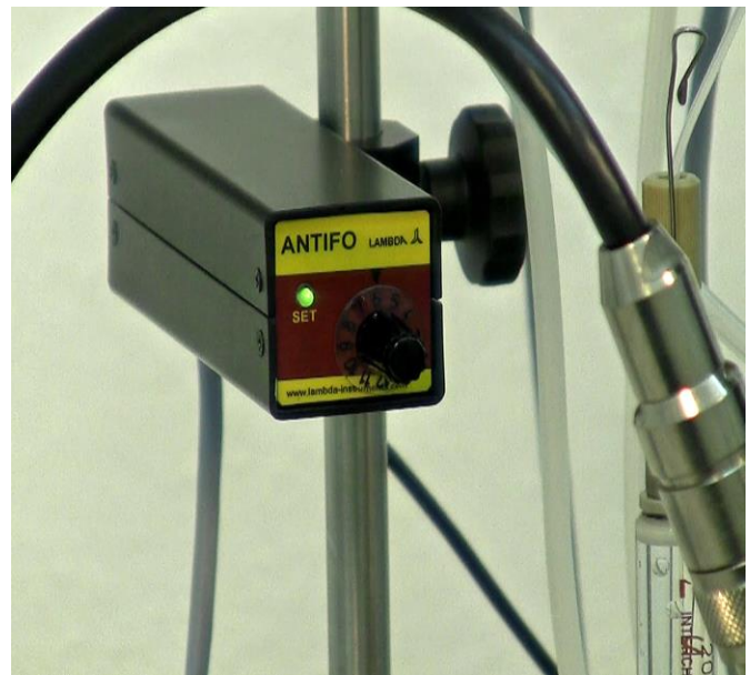
Figure 5.6—4 Sensitivity of the ANTIFO for the particular culture is now set. The LED will turn from green to yellow, when it controls the DOZITO for antifoam addition.
