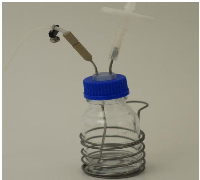
Figure 7.2—2 Clap the tubing and check that the filter is not clogged. Place the bottles in the sterilization storage bottle holder.
