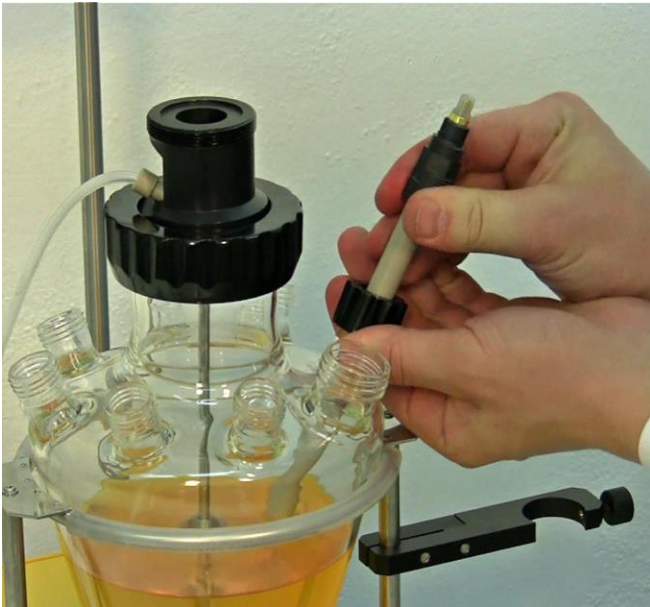
Figure 3.7—9 Insert the probe through the fixed coloured stopper and screw cap. Then, push the probe carefully into the port and adjust the height of the probe to be immersed in the medium
