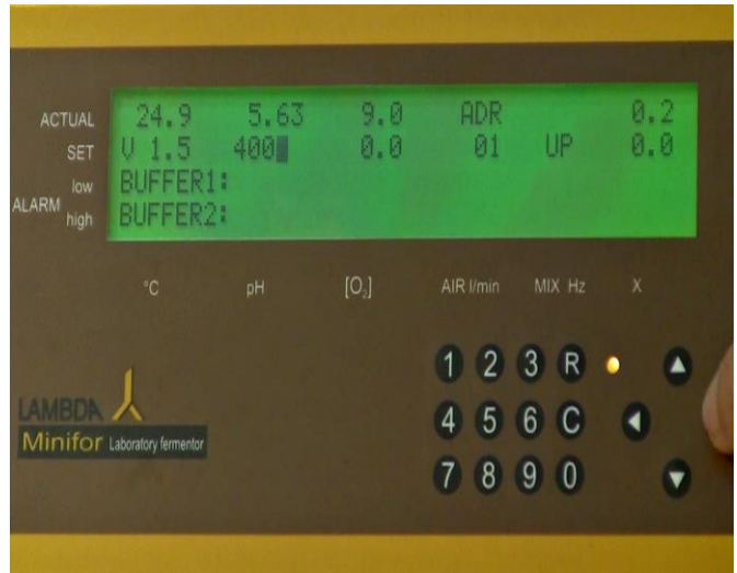
Figure 5.2—4 To start the gauging of the first pH, enter the desired pH as the set value using the number keys.
