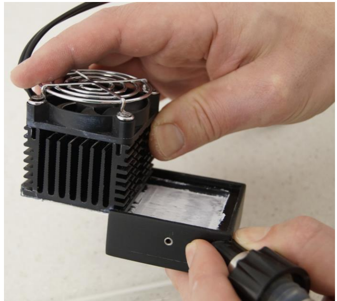
Figure 3.12—9 Attach the Peltier cooling element with control electronics and fan with the condensing finger, by placing the white surface with the thermal paste onto the respective trap in the condensing finger attachment as shown.
