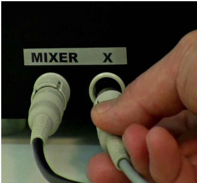
Figure 3.15—25 Connect the weighing module connection cable in the "X" socket beside the "MIXER" on the left side of the MINIFOR base control unit.
