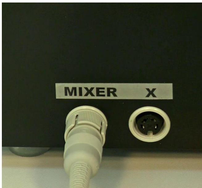
Figure 3.15—4 Connect the agitation unit cable to the "MIXER" socket present at the left side of the MINIFOR Base Unit.
