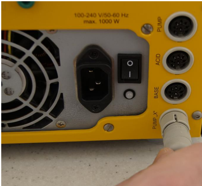
Figure 3.16—18 Feed or the Harvest pump of the weighing module should be connected to the PUMP 'X' socket.
