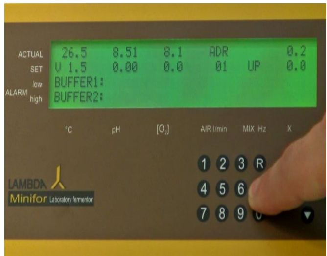
Figure 5.5—2 Long press of the calibration key “C” will activate the SET values on the display.
