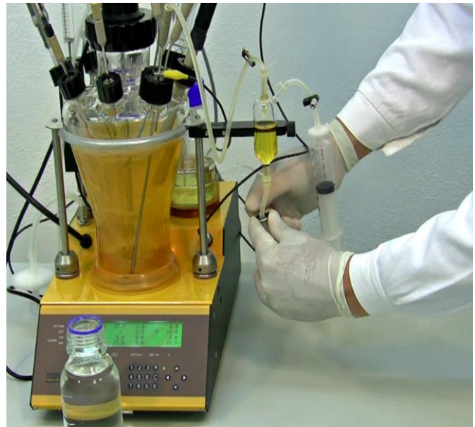
Figure 8.2—6 Open the clamp on the outlet tubing.
