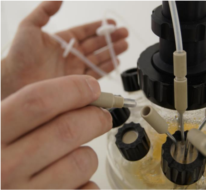
Figure 3.6—13 Connect the tubing for surface aeration to the hollow small cannula in the quadruple sampling port that stays in the head space of the MINIFOR above the medium surface.
