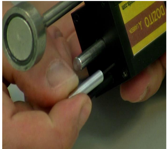
Figure 5.6—6 Insert the key at the insert point next to the pusher rod.
