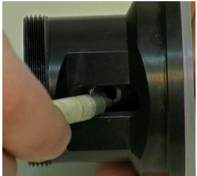
Figure 3.5—18 Insert the prepared double-seal tubing connector into the mobile cock through the head of agitation unit. Screw the double-seal tubing connector clockwise to tighten it. (ATTN: Axis of thread is 60° (please do not force it))
