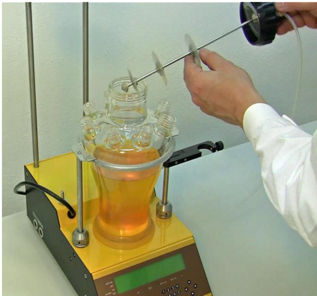
Figure 3.5—25 Place the agitation unit with the fish tails discs and microsparger into the vessel and fix the central screw cap on the reaction vessel.
