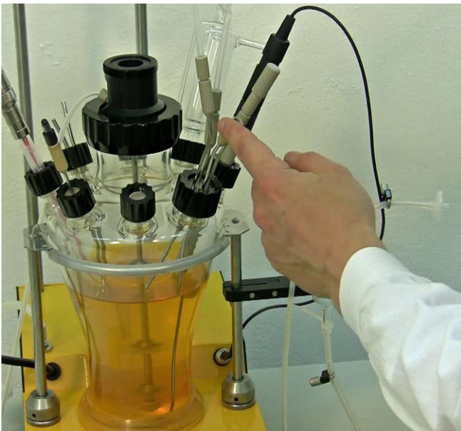
Figure 3.10—25 Remove the double-seal tubing protection closure on the longest cannula of the quadruple sampling port as shown.
