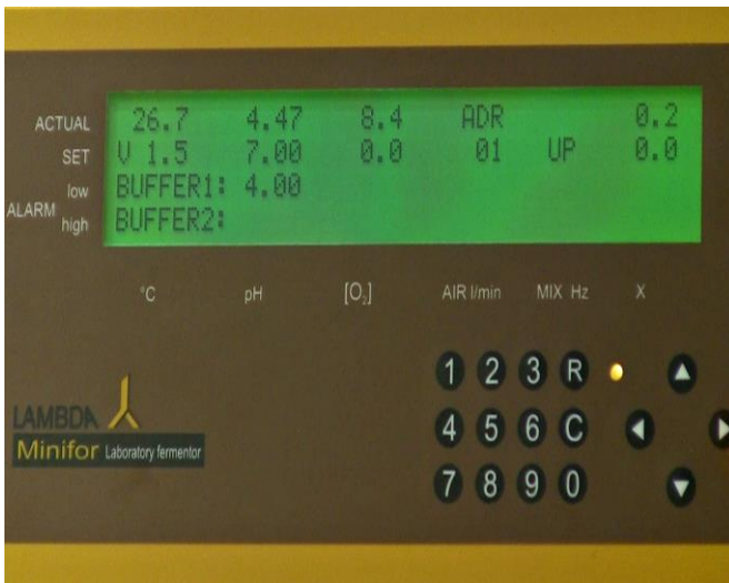
Figure 5.2—11 After pressing the right arrow key “>”, the value entered (700) will be SET as pH 7.00.
