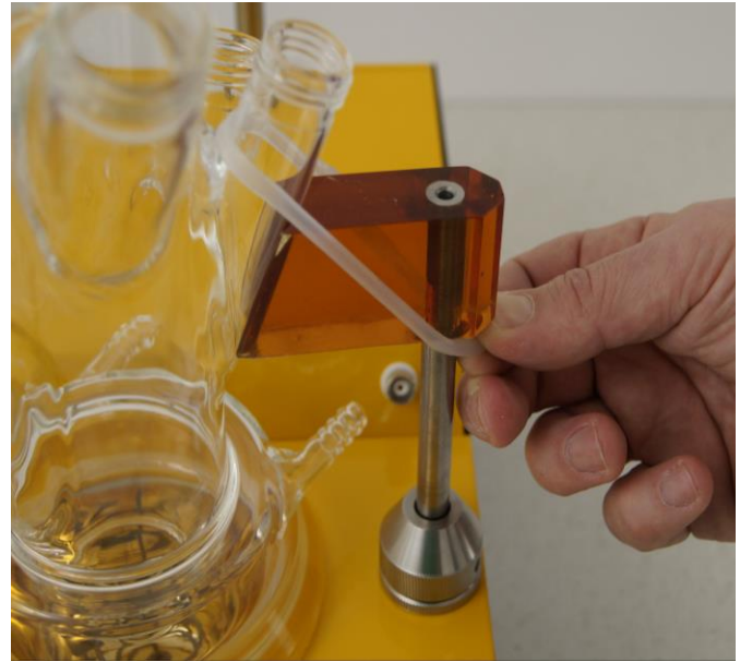
Figure 3.4—18 Pull the elastic silicone ring and affix the side arms of the vessel with the lateral reaction holder.
