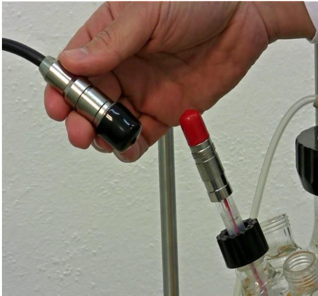
Figure 3.8—9 Take the pH probe connector from the base control unit of the MINIFOR Bioreactor. (Black cable from the base unit)
