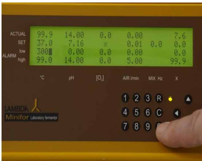
Figure 4.3—3 Move the cursor on the field of temperature minimum (ALARM LOW). Enter the desired value. If the temperature falls below this value, an alarm is activated and an asterisk is displayed on the left of the corresponding value.
