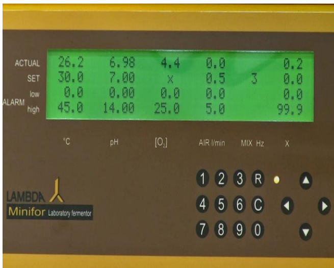
Figure 4.1—1 Stand-by mode of the MINIFOR. “R” key used to switch between Standby and Regulation state (RUN with REGULATION)
