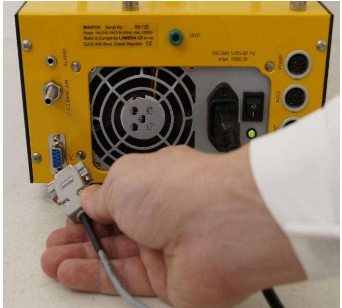
Figure 6.4—2 Connect the PC connection cable to the DB 9 connector at the rear of the base control unit.
