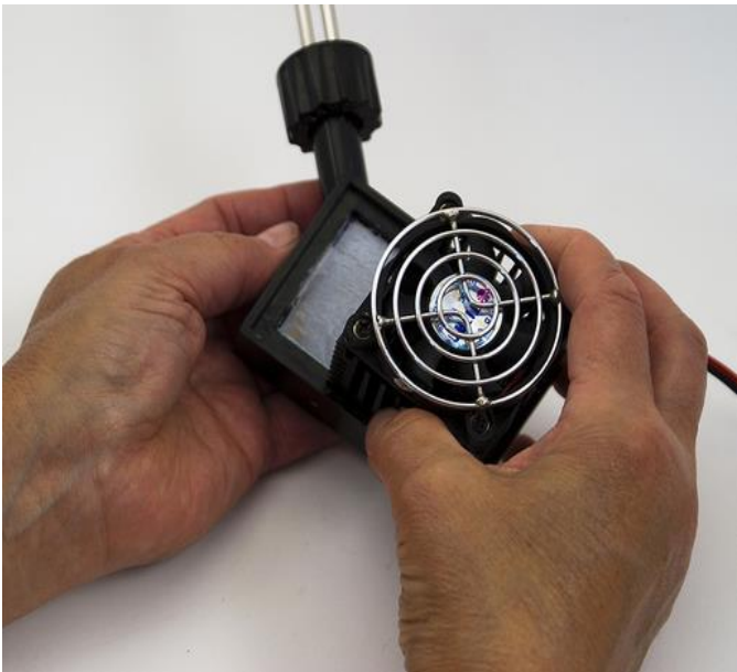
Figure 3.11—11 Attach the Peltier cooling element with control electronics and fan with the cooling loop by placing the white surface with the heat-conductive paste onto the respective trap in the cooling finger attachment as shown.
