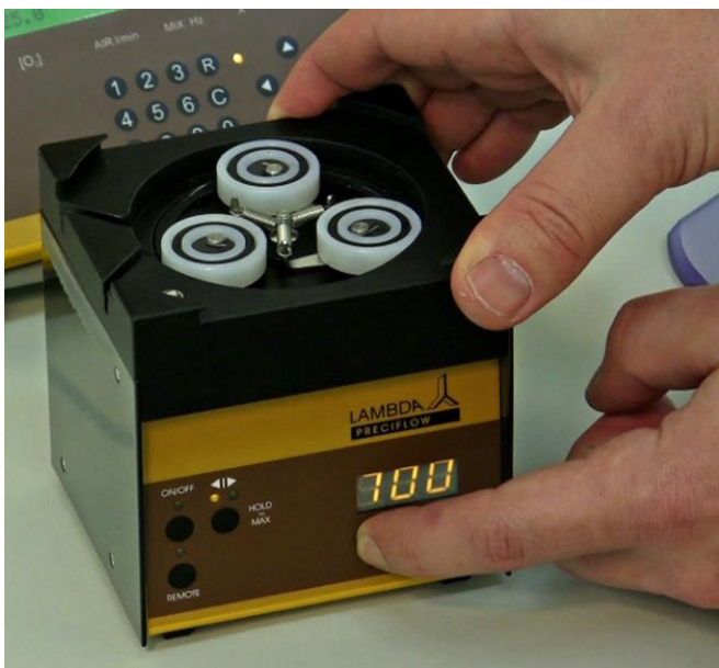
Figure 3.16—3 Set the pump speed to about 700. The speed range of about 300-700 for tubing insertion can be used.
