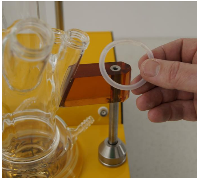
Figure 3.4—16 Place the reaction vessel on the base unit with which the distinct side arms for pH and pO 2 probes are supported by the lateral reaction holders. The elastic silicone ring helps to affix the vessel with the reaction holder.
