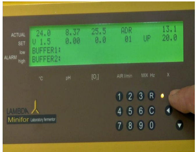
Figure 5.5—17 Use the up arrow navigation key to change from DOWN to UP.
