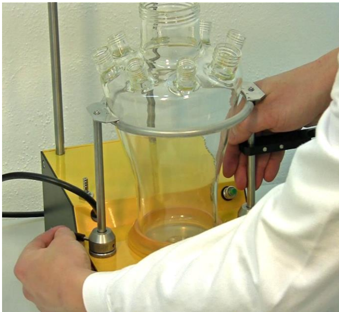
Figure 3.4—11 While supporting the reaction vessel holder with one hand, tighten around the slots of the reaction vessel holder with the given key.
