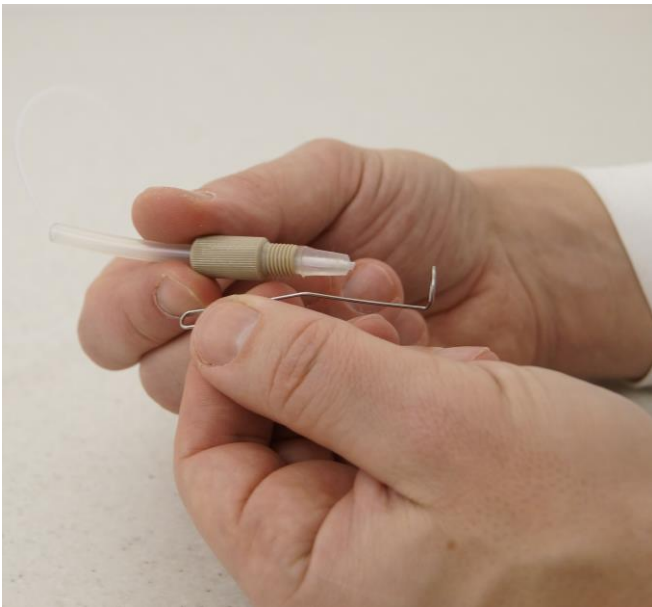
Figure 3.14—9 Insert the holder for autoclaving to the threaded neck of the double seal PEEK fitting part.
