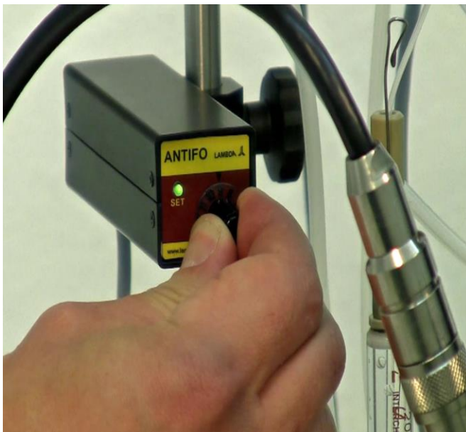
Figure 5.6—3 Now rotate the knob anticlockwise (about 1mm) to set the sensitivity point and the LED displays green i.e. the point at which yellow turns to green.
