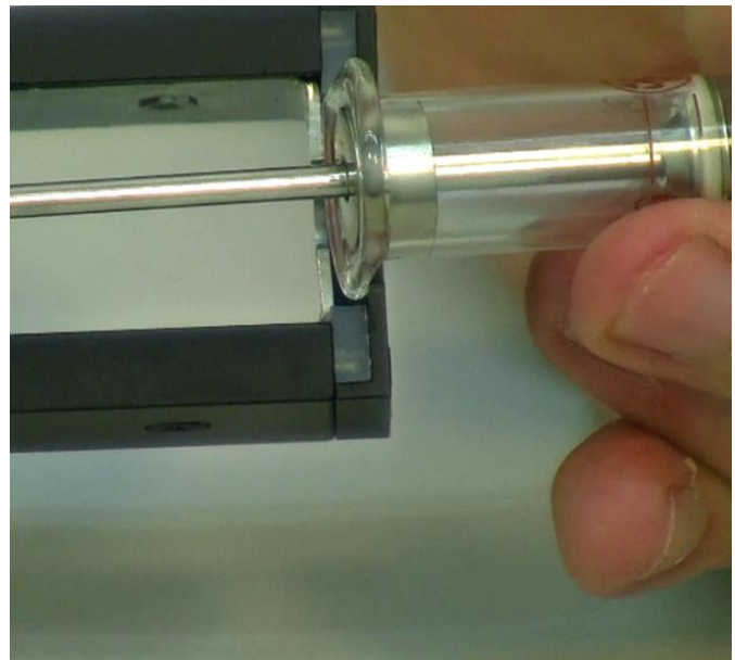
Figure 3.14—20 Place the bottom of the syringe into the syringe pump fixing slot on the DOZITO pump as shown. Rotate the DOZITO pump by holding the syringe firmly, to make the syringe fit on its position.
