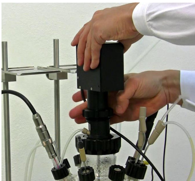
Figure 3.15—3 Once the magnets are engaged, the air-input with the mobile PEEK cock displace downwards. Secure the vibromixer firmly by screwing the cap.
