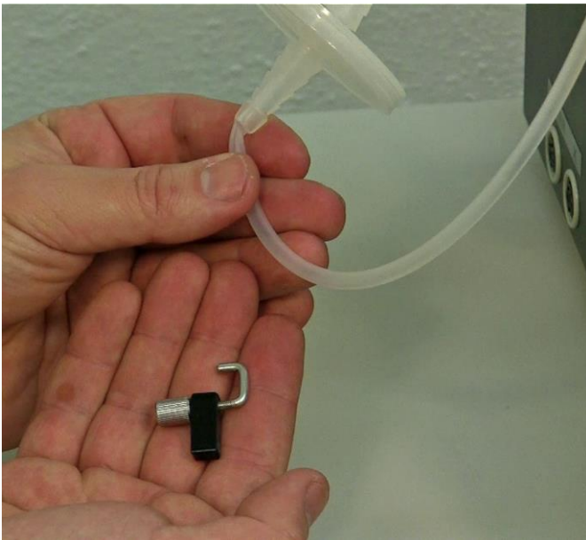
Figure 3.6—7 The safety lock is provided for the air input. This protects the air-input filter for liquids entering the air-output / air-input line).
