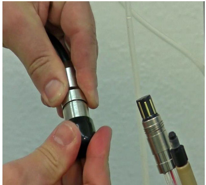
Figure 7.1—8 Protect the female cable connector using a cap against contamination.
