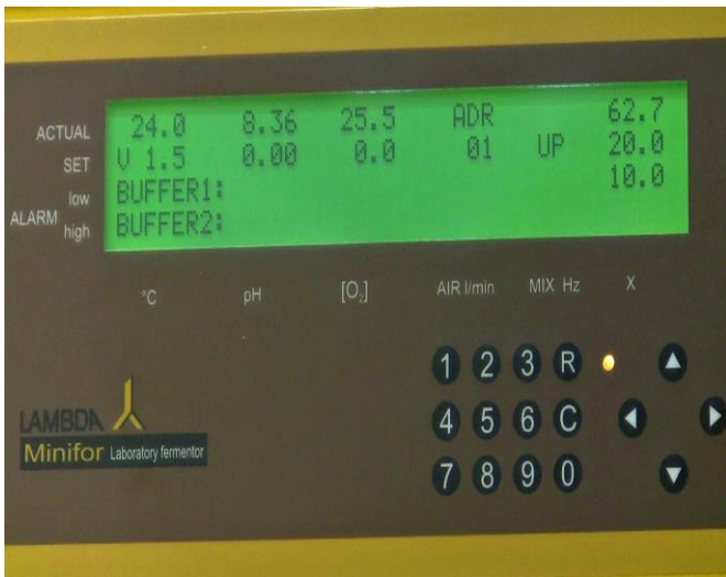
Figure 5.5—11 The entered 200 will appear as 20.0 in the SET value after pressing the right arrow key (>).
