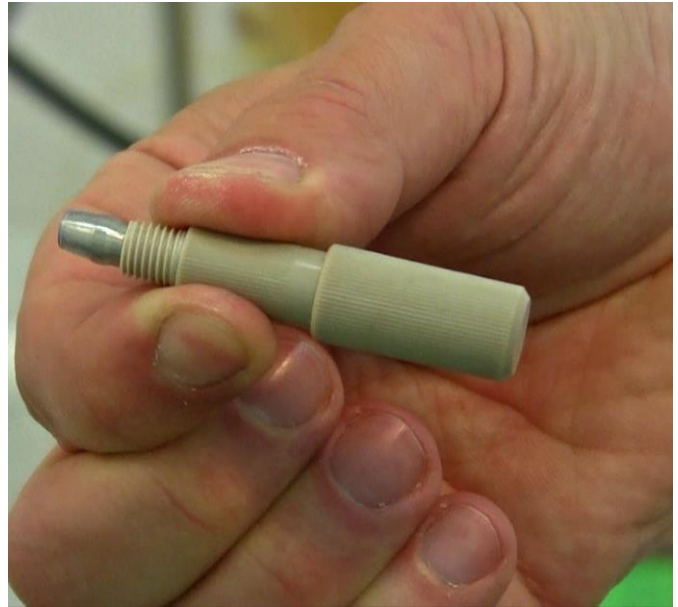
Figure 3.10—16 Complete set for inoculation. The free end with the double seal conical insert has to be inserted on one of the cannulas or needles from the quadruple sampling port.
