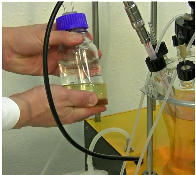
Figure 3.10—30 Stock bottles can be conveniently kept at the back of the MINIFOR base control unit using the magnetic bottle holder.
