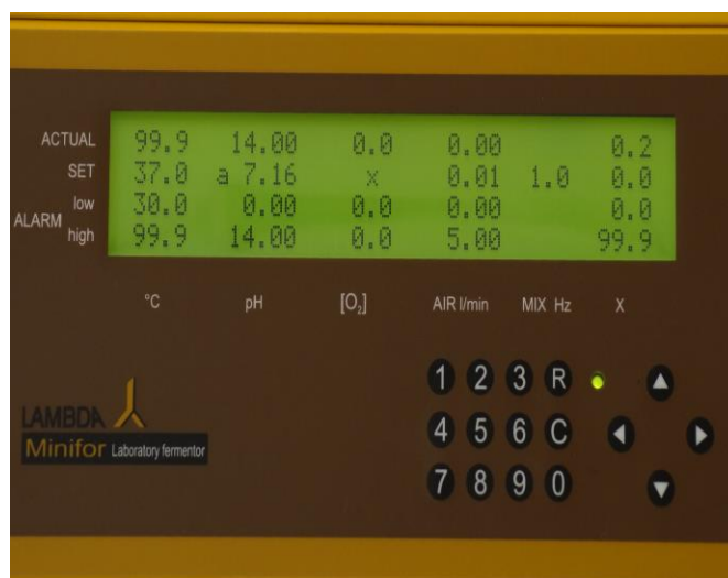
Figure 4.2—2 Regulation / Operation mode - The regulation is activated by pressing key "R" and the LED turns to green. The display shows the measurement of all the parameters.
