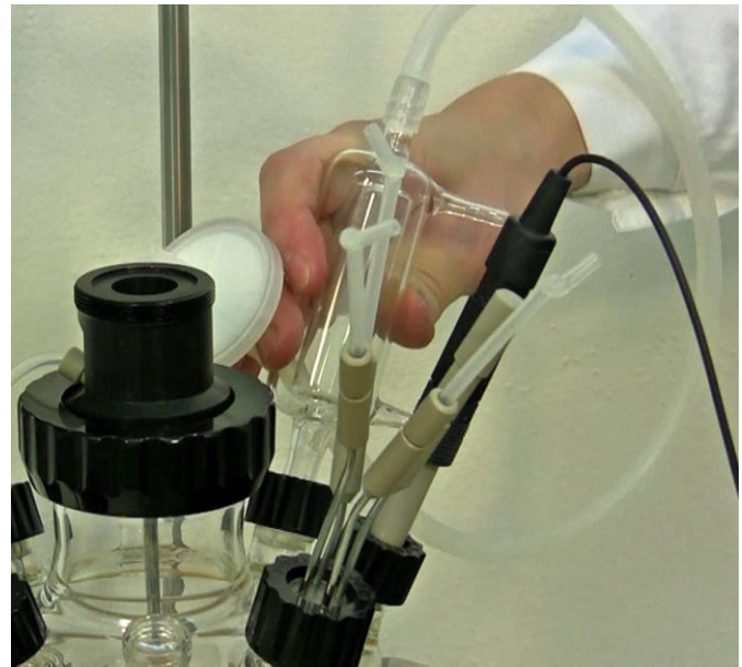
Figure 3.12—3 Insert the outgas condenser into the port with the open stopper, washer and black screw cap. Select a port that will not be disturbed during the work.
