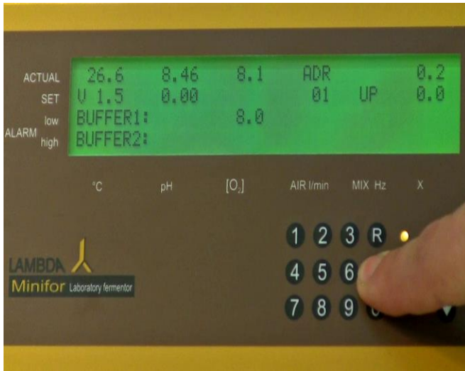
Figure 5.3—7 Press the calibration key "C". The calibrated value will be shown as BUFFER 1 value of [O 2 ].
