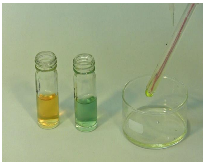
Figure 5.2—18 Rinse the probe with deionised water and dry it with the blotting paper.
