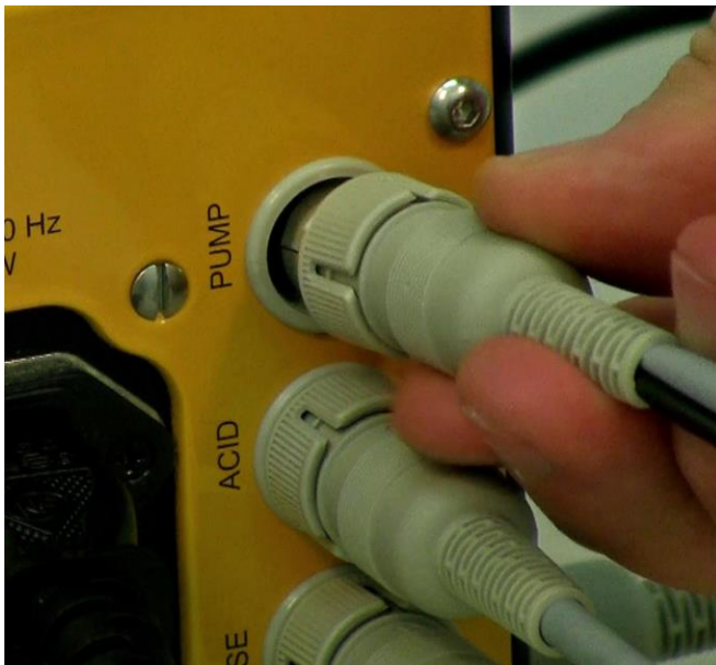
Figure 3.14—25 Connect the ANTIFO cable (8 poles) to the "pump" socket present on the rear of the MINIFOR base control unit.
