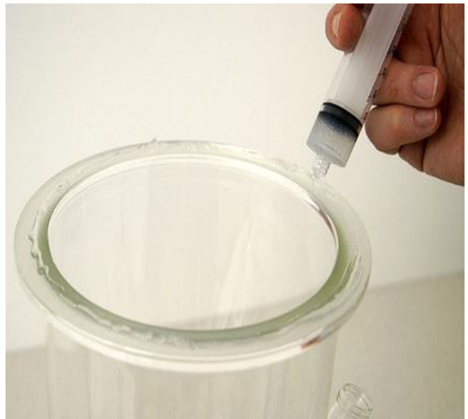
Figure 3.4—24 Apply the mixture on the whole circumference of the lower vessel part's brim like a "spaghetti".
