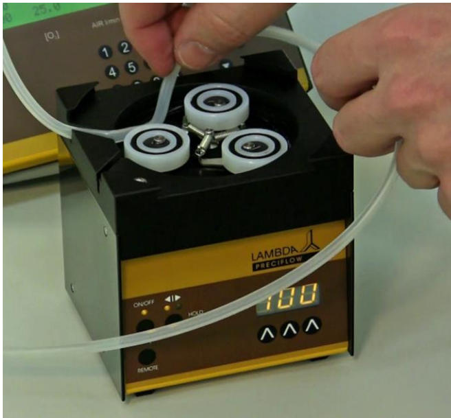
Figure 3.16—5 Press the tubing into the back slot on the top of the peristaltic pump. Thin tubing should be pushed completely to the bottom of the slot.
