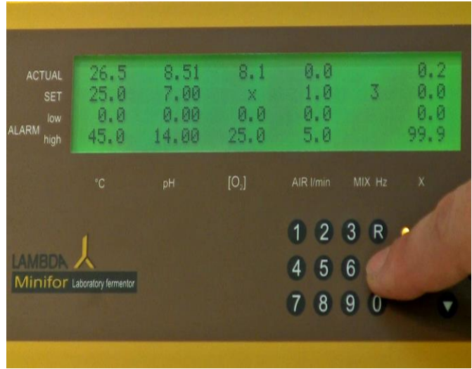
Figure 5.3—2 Make sure that the agitation value entered as SET value. Press the calibration key “C”. (Please note that the agitation of the medium take place even in the calibration mode).
