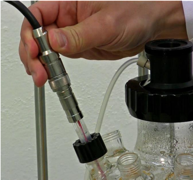
Figure 3.15—7 Connect both the pH probe connector cable from the MINIFOR base unit with the pH probe. Rotate and adjust the connector cable for exact locking of grooves.
