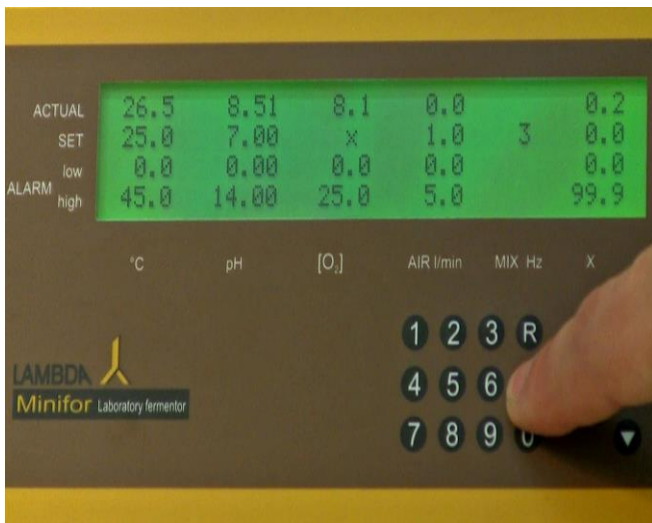
Figure 5.5—1 When the vessel is well positioned on the scale module, press the calibration key “C” to change the standby mode to the calibration mode.
