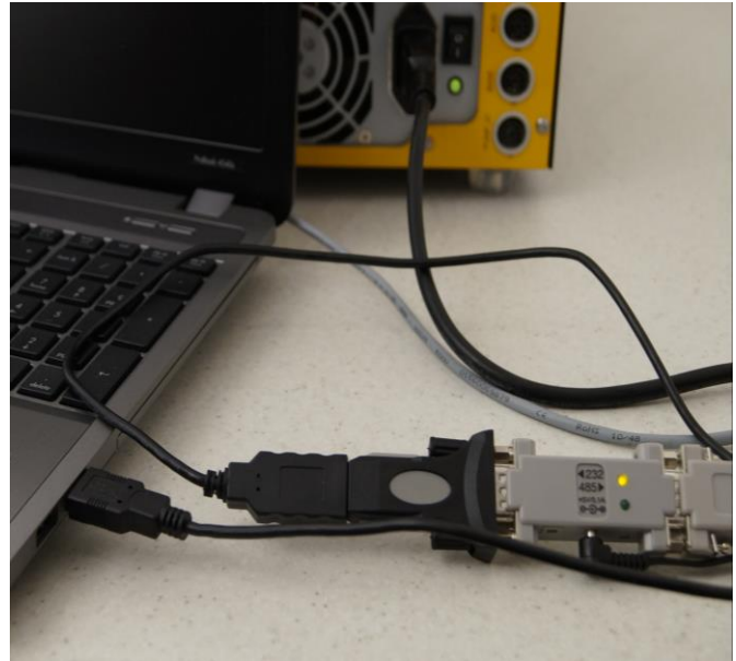
Figure 6.4—6 The PC connection cable along with the RS converter is connected to the PC with the help of the USB connector.
