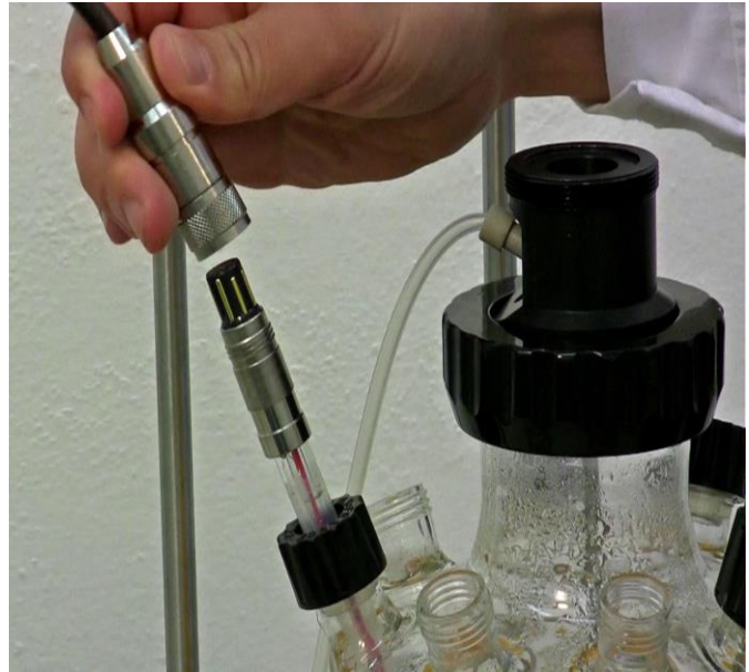
Figure 3.8—10 Remove the black protection cap on the sensor (top part) of the cable and red protective cap from the pH probe.
