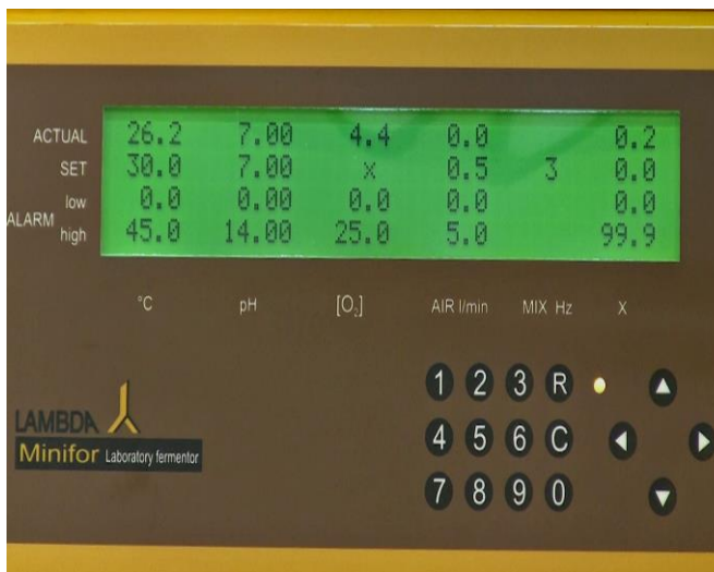
Figure 5.2—20 The ACTUAL value of the parameter pH should be 7.00 (It can range between 6.95 – 7.04)
