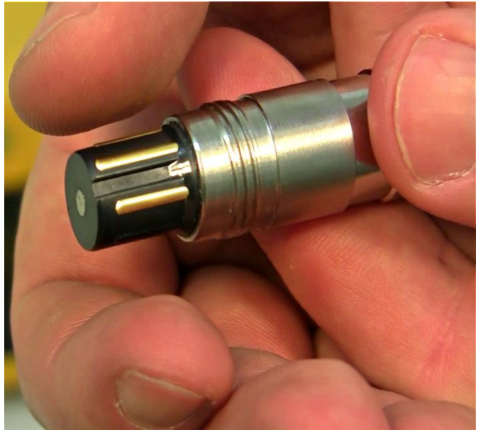
Figure 3.8—2 Care should be taken not to touch the sensor part of the probe.
