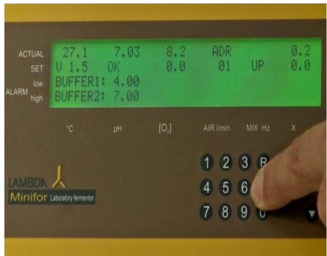
Figure 5.2—14 Once the value becomes stable, press the calibration key “C”. The calibrated value will be saved and displayed as BUFFER 2 pH value.
