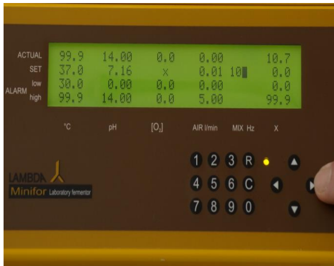
Figure 4.3—5 Move the cursor using the navigation key and place it on the MIX Hz column. Set the desired frequency of agitation using the number keys and press the right arrow for saving the entered value.
