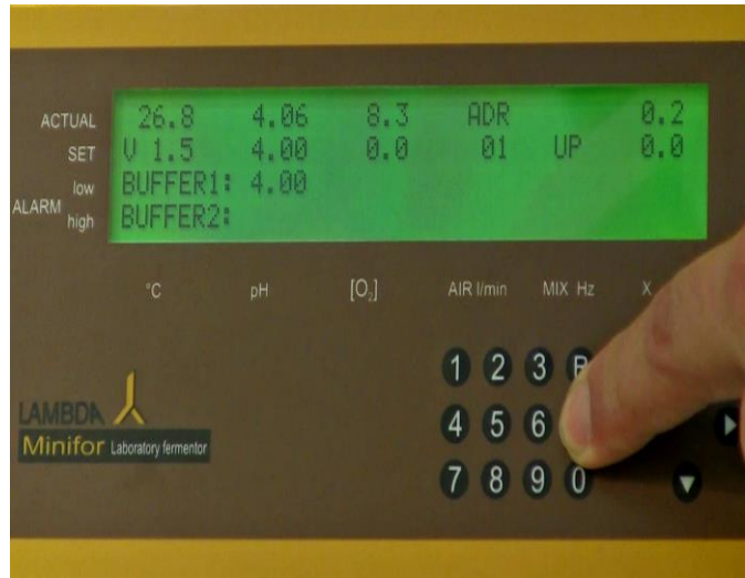
Figure 5.2—8 Once the ACTUAL value of the pH is stable, press the calibration key "C" in order to save the calibration. The calibrated value will be displayed as BUFFER 1 value of pH.
