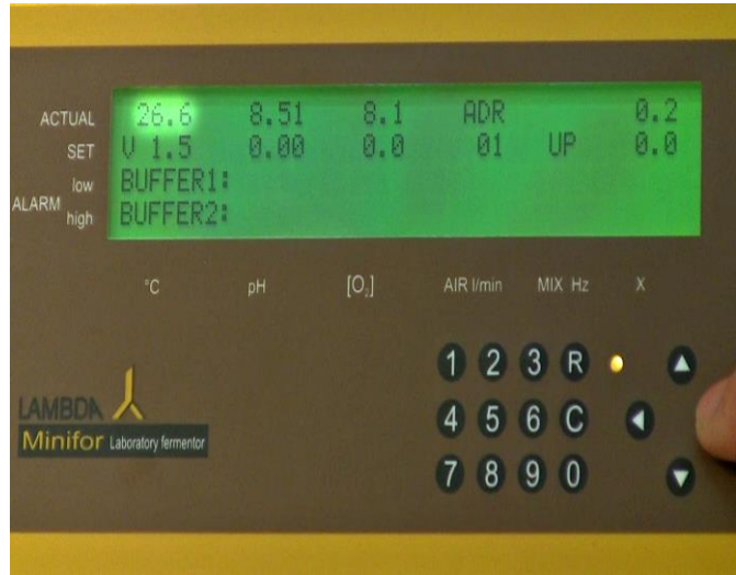
Figure 5.3—4 Check the highlighted ACTUAL value of the temperature (this should be the desired temperature for the run). Refer the corresponding Oxygen saturation value for the temperature in the table 5.3.4 Oxygen saturation in water. [e.g. oxygen saturation in water at 26.5°C = 8.0 mg O 2 /l]
