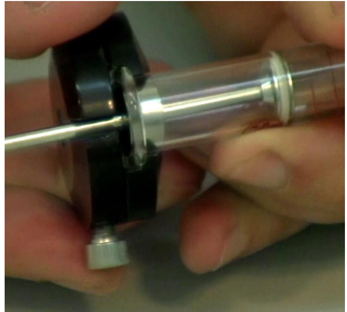
Figure 3.14—13 Insert the syringe bottom to the black syringe holder.
