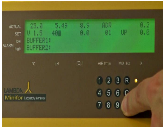
Figure 4.1—8 Changing the value of the selected parameter using number keys.
