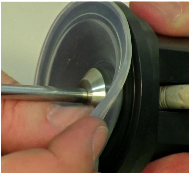
Figure 3.5—19 Ensure that the large silicon sterility membrane is fitted correctly and firmly in the designed grooves on the head of the agitation unit.
