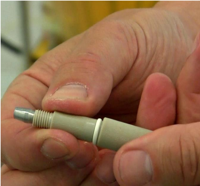
Figure 3.10—15 Fix the septum protection cap on the threaded side of the white septum O-ring.
