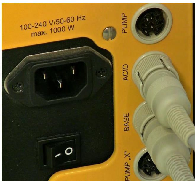
Figure 3.15—14 Connect the Peristaltic pump that regulates the acidity of the reaction to the “ACID” socket at the rear of the MINIFOR base control unit.
