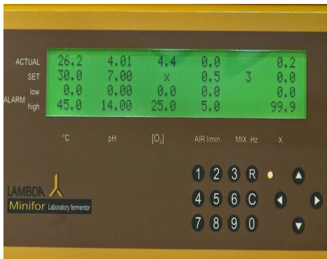
Figure 5.2—23 The ACTUAL value of the parameter pH on the display should be 4.00 (It can range between 3.96 – 4.04)
