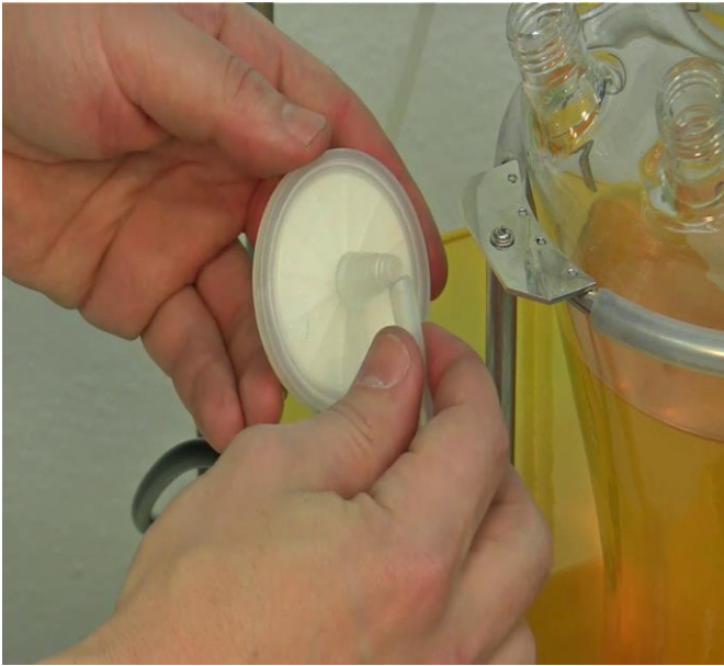
Figure 3.6—5 Connect a small piece of tubing (cut as desired) to the shown free end of the air-input filter.
