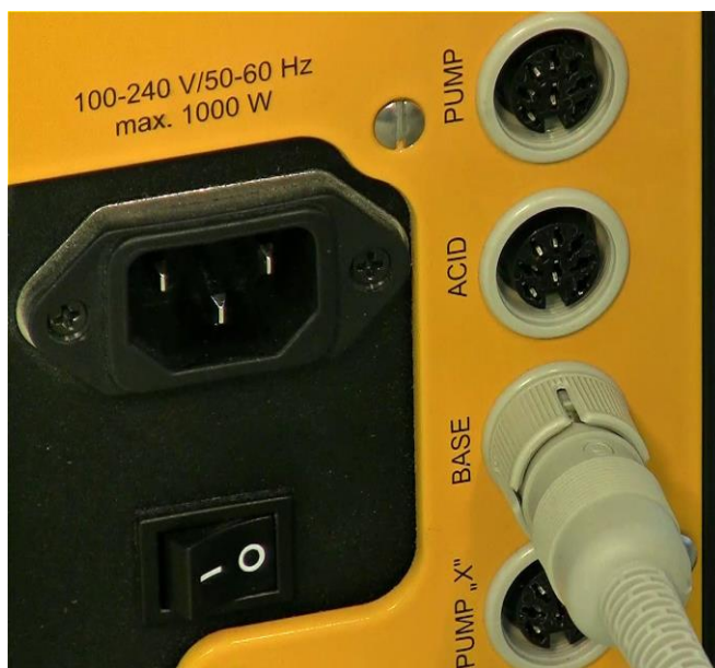
Figure 3.15—13 For automatic pH control, connect the pump / Massflow that controls alkalinity of the reaction to the “BASE” socket at the rear of the MINIFOR base control unit.
