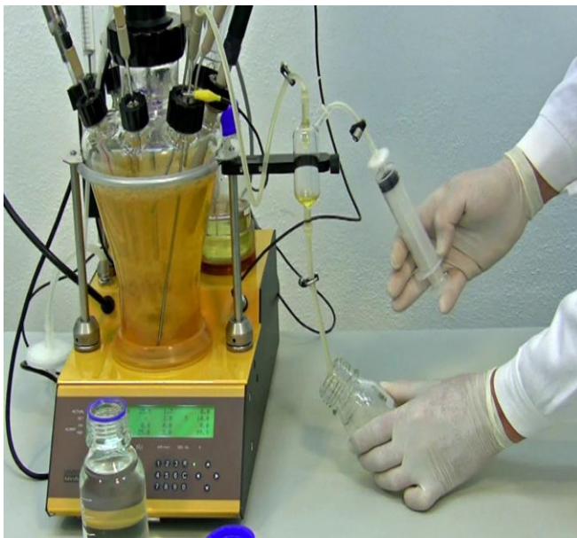
Figure 8.2—7 Use a beaker / bottle to collect the flushed waste sample. Push the syringe plunger to pass the air drawn into the sampling device and thus making the flow of the flushing liquid from the sampling device into the wastage bottle.
