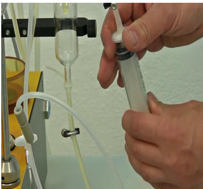
Figure 7.1—11 Remove the syringe from the sterile sampling device. Close all the tubing clamps. If the sampling device is used then remove and disconnect it from the cannula and syringe.
