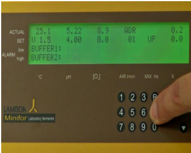
Figure 5.2—3 Continuous pressing of "C" key will activate the cursor of the set value of pH.
