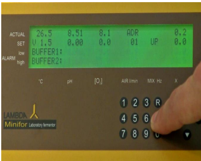
Figure 4.1—4 Press the "C" - calibration key continuously to activate the cursor.
