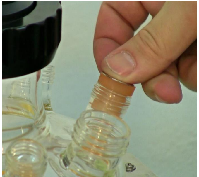
Figure 3.7—6 Make sure the washer is placed on to the rubber stopper.
