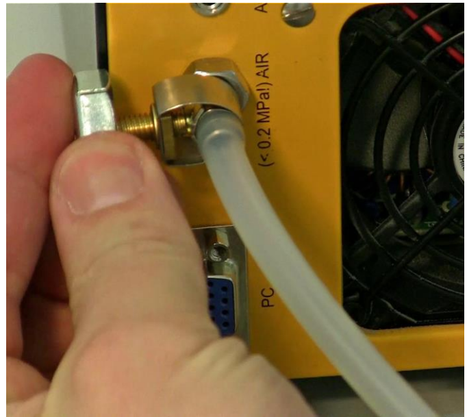
Figure 3.15—22 Secure the connection using the valve.
