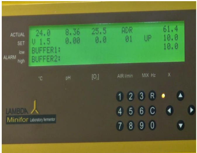
Figure 5.5—8 Once calibrated, the initial value will appear as BUFFER 1 value of the parameter “X”.
