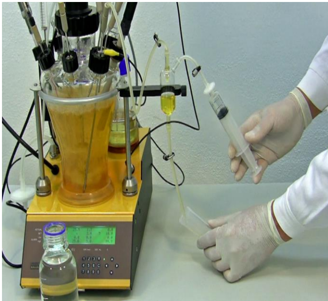
Figure 8.2—11 Push the syringe plunger to pass the air drawn into the sampling device and thus making the flow of the flushing liquid from the sampling device into the sterile sampling tube. Secure the sampling tube with a cap.
