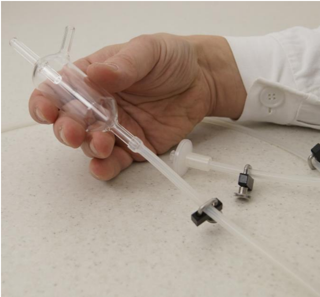
Figure 3.10—19 Silicone tubing which is 10 - 20 cm long needs connected to the output arm provision on the glass device i.e. the vertical arm opposite to the inlet sampling connection with the Bioreactor (on the lowest part of the device)
