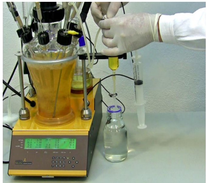
Figure 8.2—4 Close the clamp on the inlet tubing to avoid the back flushing of the sample into the reaction vessel.
