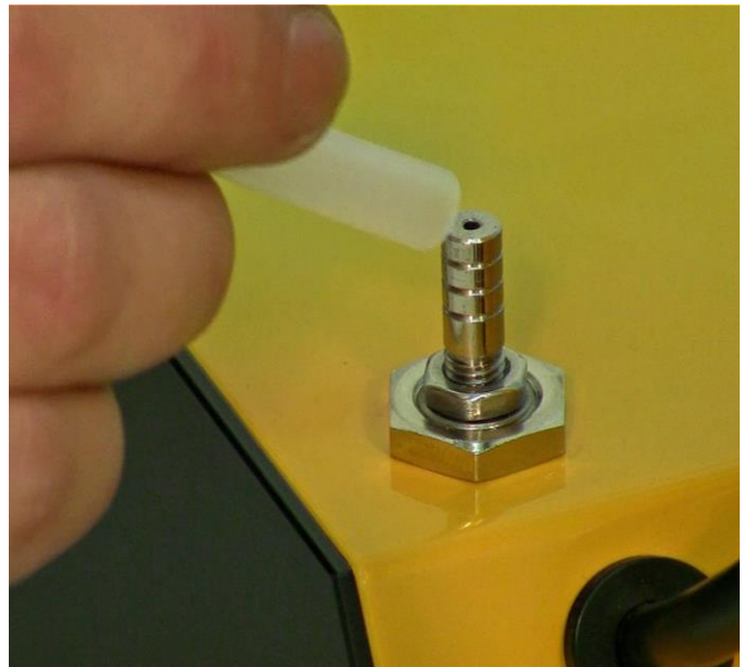
Figure 3.6—6 With the other end of the tubing from the air-input filter, connect it to the air outlet on the base control unit as shown. Insert the tubing deeply till the bottom of the air outlet.
