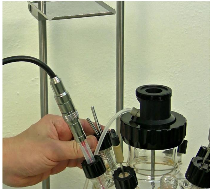
Figure 3.11—4 Secure and fasten gently with the black screw cap.
