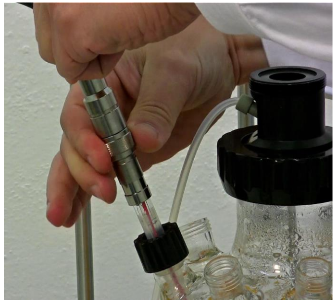
Figure 3.8—12 After locking the grooves of the pH probe and connector cable, tighten the connection by screwing the threaded lock on the connector cable by rotating as shown.
