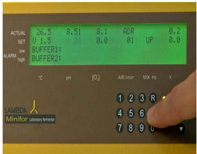
Figure 4.1—5 The cursor is represented by the blinking of the activated digit.
