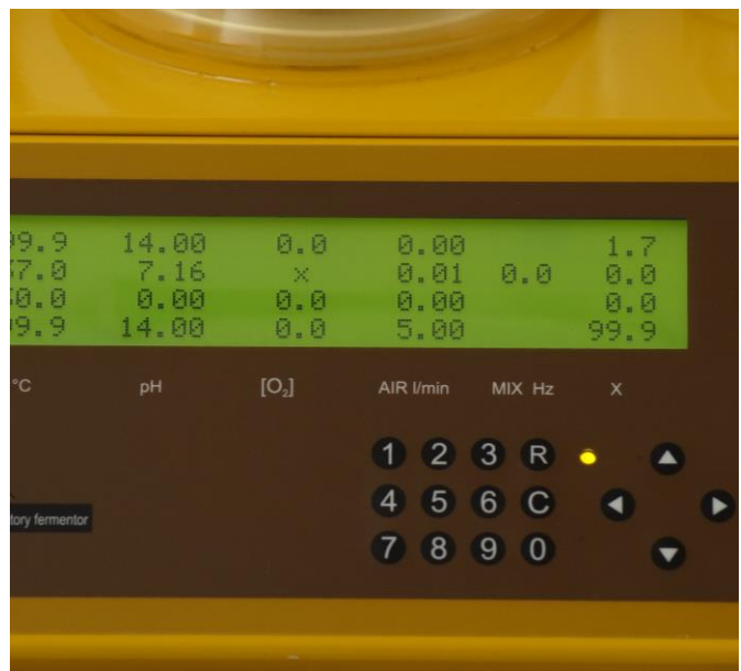
Figure 3.15—45 When switched on, the MINIFOR starts with a beep sound and yellow LED display on the control panel. This represents the Stand-by mode of the MINIFOR fermentor-bioreactor.
