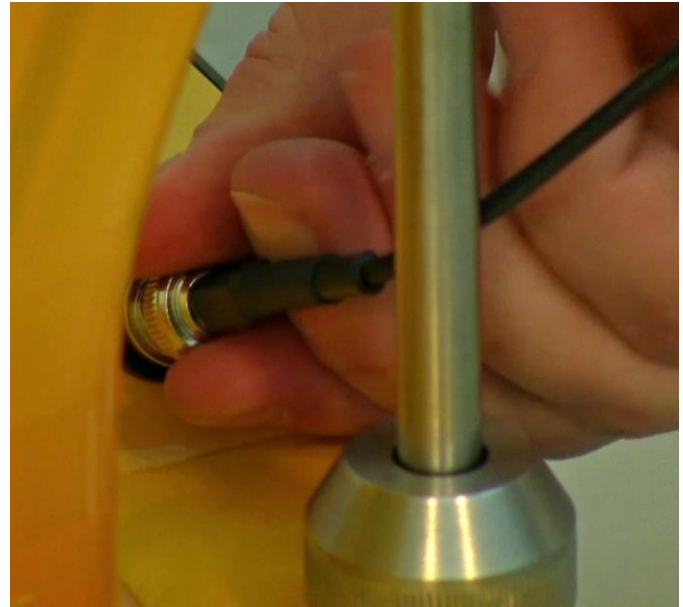
Figure 3.15—20 Secure the pO 2 (DO) probe connector into the socket by rotating and pressing to lock it together.
