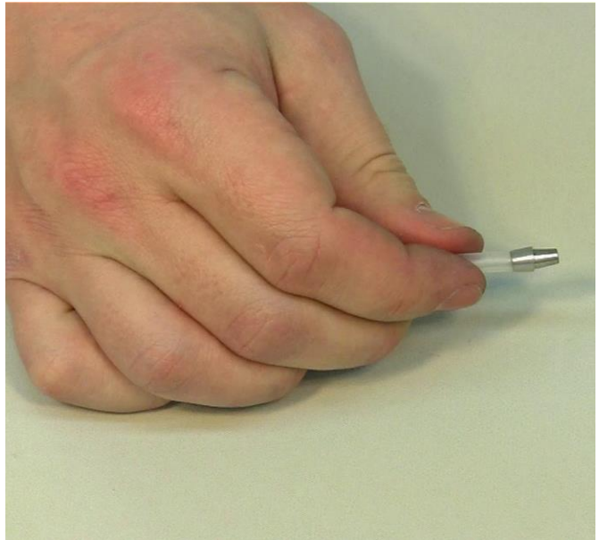
Figure 3.10—8 The resulting double-seal conical insert with the tubing should be like in figure i.e. half the portion of the conical insert can be found inside the tubing.
