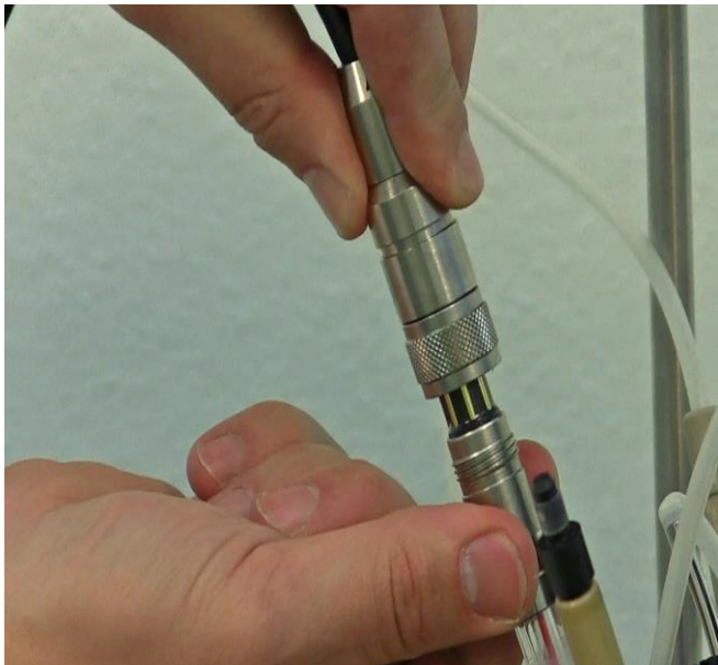
Figure 7.1—7 Disconnect the pH probe connector from the pH probe.
