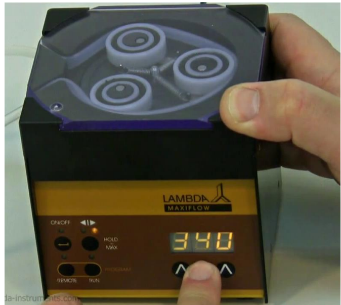
Figure 3.16—11 Each \wedge \wedge \wedge arrow can be used to change the corresponding digit on the flow rate.
