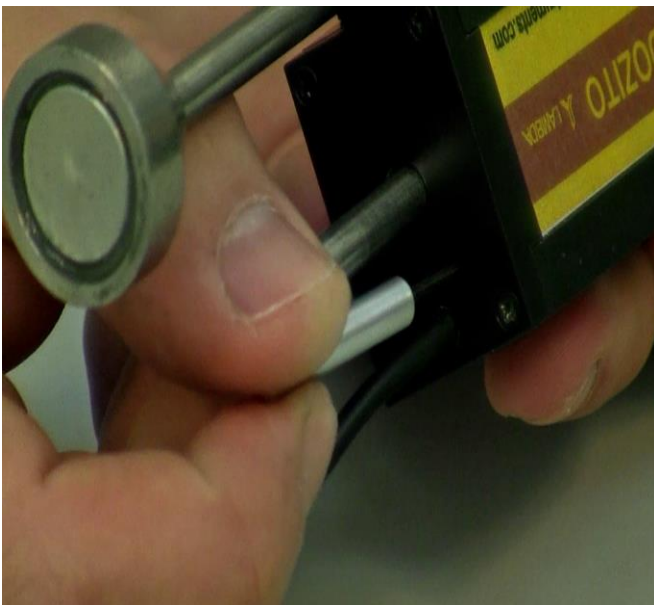
Figure 5.6—7 Screwing in = clockwise rotation = decrease of the delivered anti-foam volume / step
