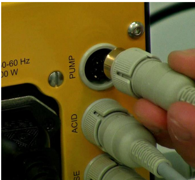
Figure 3.11—15 Connection for the Peltier cooling device: on the rear of the MINIFOR.
