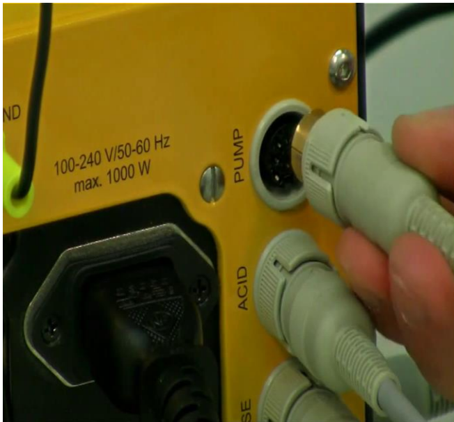
Figure 3.15—23 Peltier outgas condenser can be directly connected on the “PUMP” socket present at the rear of the MINIFOR base control unit.
