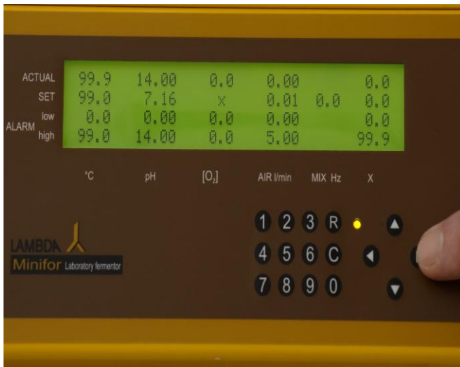
Figure 4.3—1 Move the cursor by using arrows on the field for the temperature setting (SET °C, second row, first column).
