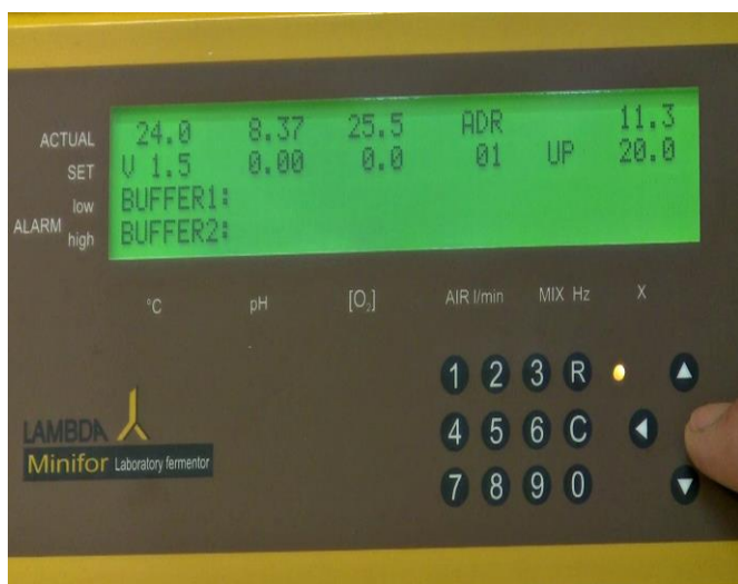
Figure 5.5—18 Press the right arrow navigation key to save the value, once the regulation of pump is selected.
