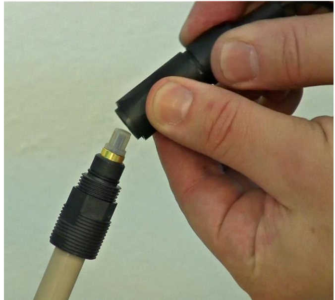
Figure 3.15—16 Adjust the sleeve of the pO 2 (DO) probe connector by pushing it up as shown.
