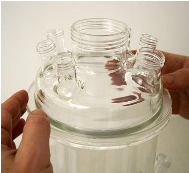
Figure 3.4—27 Place the upper part onto the lower vessel part. The paste fills any cavity between the joining surfaces and is completely gas tight and also does not generate any stress in the glass.
