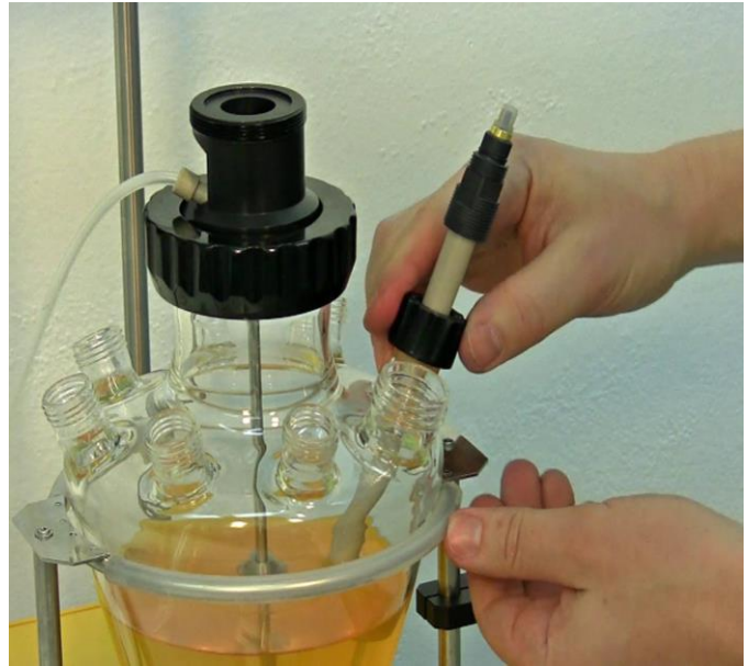
Figure 3.7—10 Tightly secure the black screw cap placed on the top of the coloured stopper.
