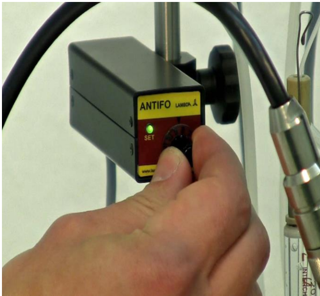
Figure 5.6—1 Once the connections are made, the ANTIFO LED will be illuminated as green.
