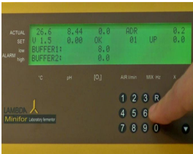
Figure 5.3—12 Press the calibration key "C". The calibrated value will be saved and displayed as BUFFER 2 value of [O 2 ]. OK message will be displayed if the calibration done correctly.
