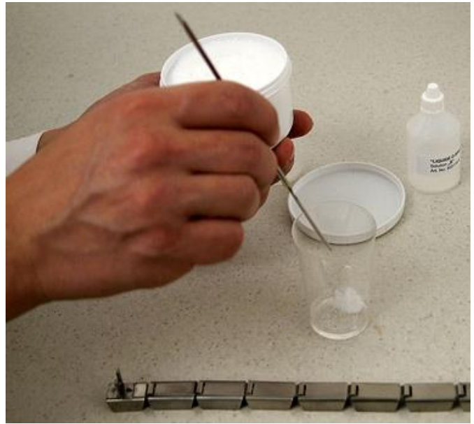
Figure 3.4—22 Take equal parts of solution A and solution B in a non-glass beaker. For example: 2g of Solution 'A' and 2g of Solution 'B'. Aerosil powder is added in such an amount until the mixture is no more flowing.
