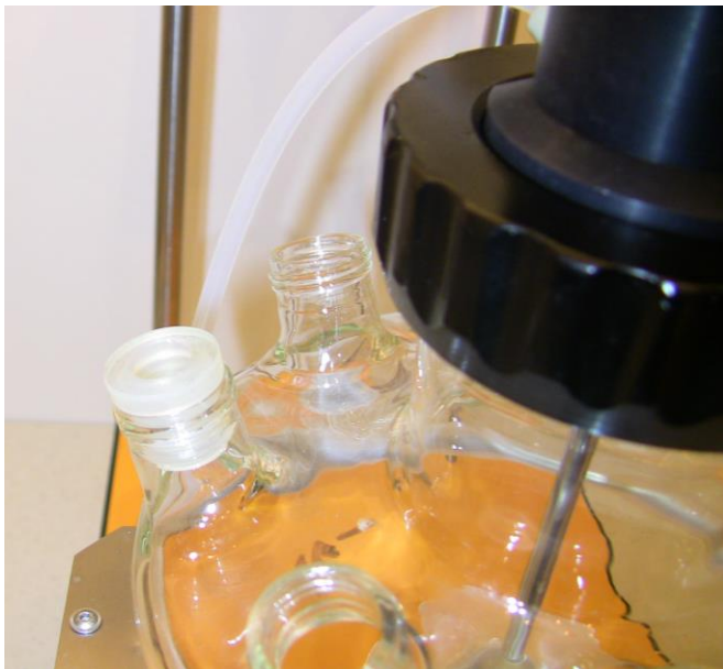
Figure 3.8—3 Place any one of the provided white open stopper on the port which is opposite to the pO 2 probe port.
