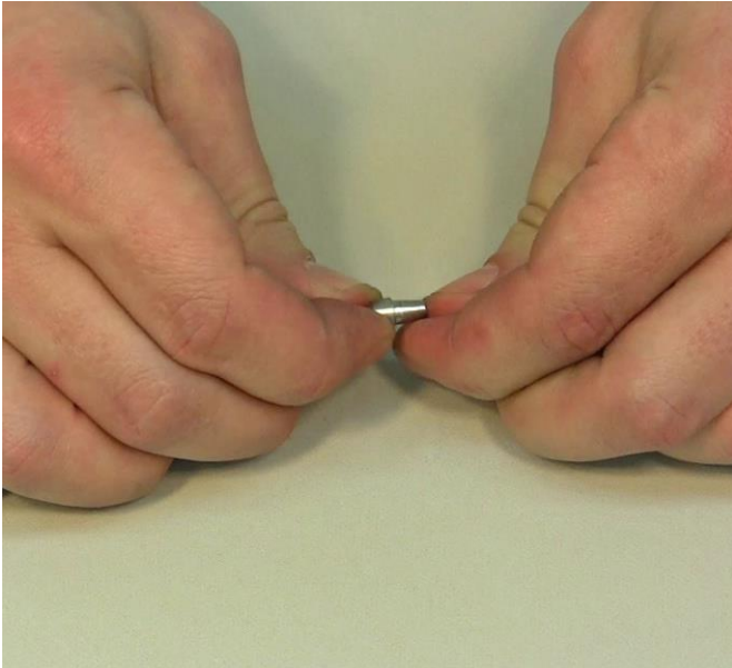
Figure 3.5—7 Insert the double-seal conical insert into the tubing which is freely flowing on the other side of the PEEK fitting.
