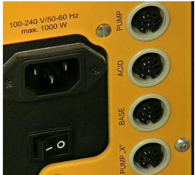
Figure 3.16—15 Pumps has to be connected into the respective sockets at the rear of the MINIFOR base control unit.
