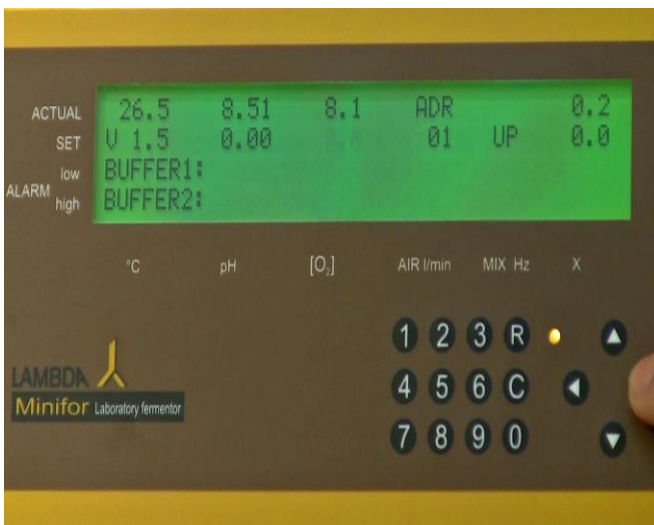
Figure 4.1—6 Once the cursor is activated after the long press of "C" key, pressing the arrows will move the cursor to the corresponding direction.
