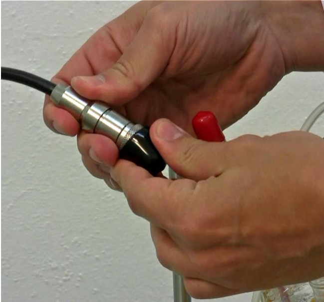
Figure 3.15—5 Take the pH probe connector from the base unit of the MINIFOR Bioreactor. (Black cable from the base unit). Remove the black protection cap on the sensor (top part) of the cable.
