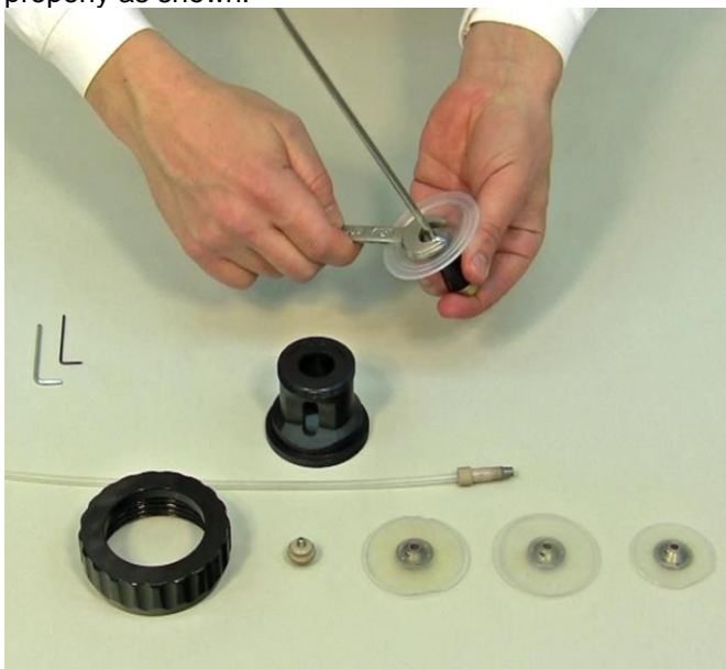
Figure 3.5—15 Securely tighten the nut at the concave side of the silicone sterility membrane which in-turn firmly holds the mobile cock with the membrane.
