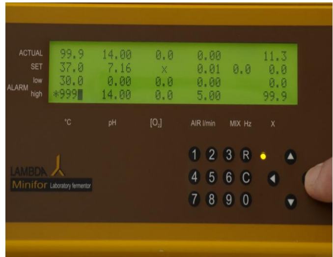
Figure 4.3—7 Alarm can be deactivated by changing the alarm high value and by taking needed precautions to maintain the temperature.
