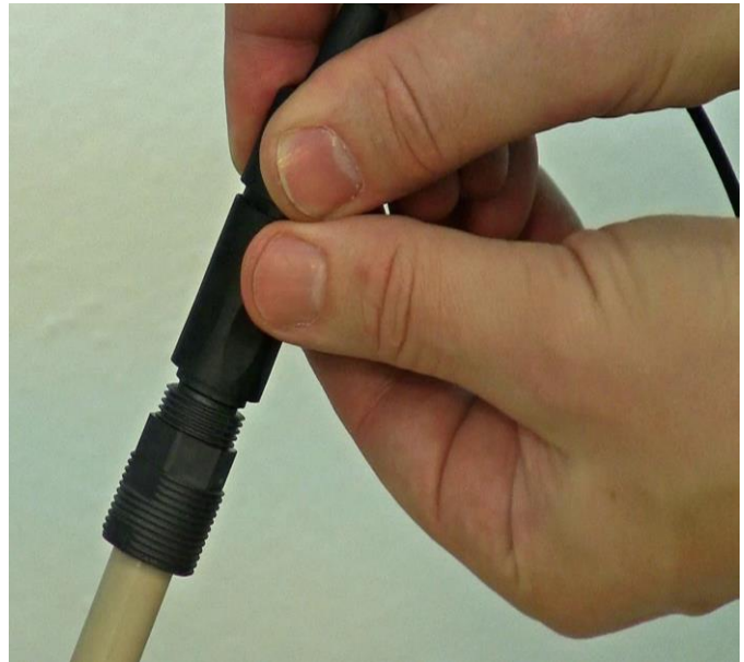
Figure 3.7—12 Place and adjust the pO 2 (DO) probe connector by rotating to find the position for exact locking of grooves with the pO 2 (DO) probe.
