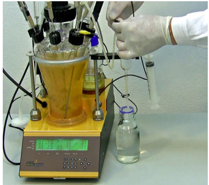
Figure 8.2—2 Open the clamp on the sampling inlet (i.e. Between the MINIFOR and the sampling device)
