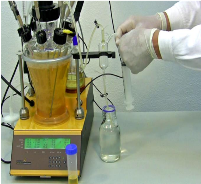
Figure 8.2—13 Once the sampling is done, place the outlet tubing into the 70% Ethanol solution and close all the clamps in the sampling device.
