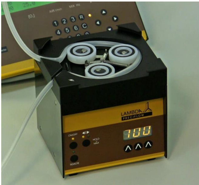
Figure 3.16—7 Press the tubing into the front slot to secure it.
