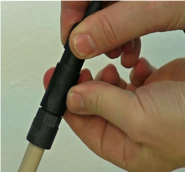
Figure 3.7—13 After fixing the pO 2 (DO) probe and connector exactly in locking position, push down the sleeve of the pO 2 (DO) probe connector and secure it sufficiently with screw fitting.
