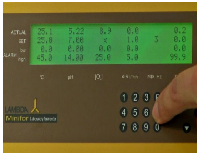
Figure 5.2—2 Change the stand-by mode into calibration mode by pressing the calibration key "C".
