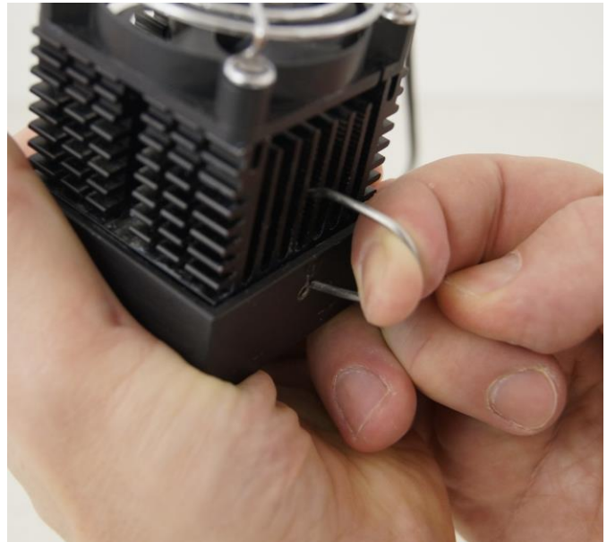
Figure 3.12—11 Locking clamp has to be pulled firmly through the Peltier cooling element with control electronics and fan and fixed into the hole on both sides of the cell, to make the Peltier cooling finger intact.
