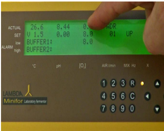
Figure 5.3—10 The ACTUAL reading for dissolved O 2 should always be '0' when the probe is disconnected. (If this is not the case then the probe may be faulty and you should check chapter Polarization, exchange of pO 2 Membrane / liquid, cleaning or contact the Lambda Helpdesk).
