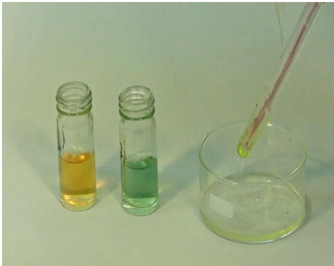
Figure 5.2—9 Wash the probe with deionised water and dry it with the blotting paper.
