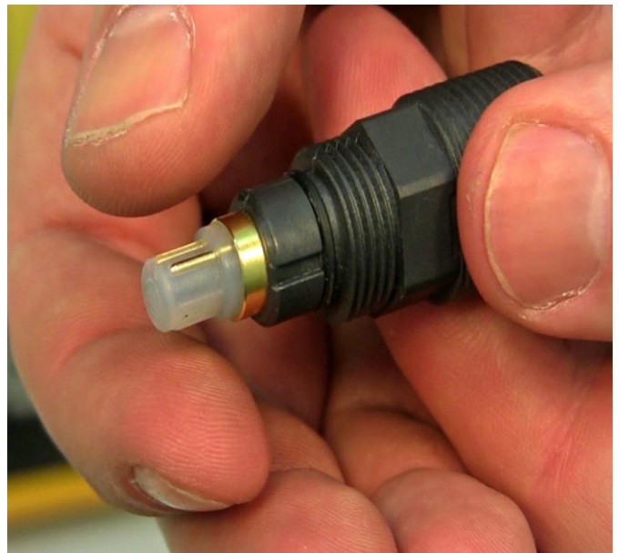
Figure 3.7—4 Please be careful not to touch this part of the probe.
