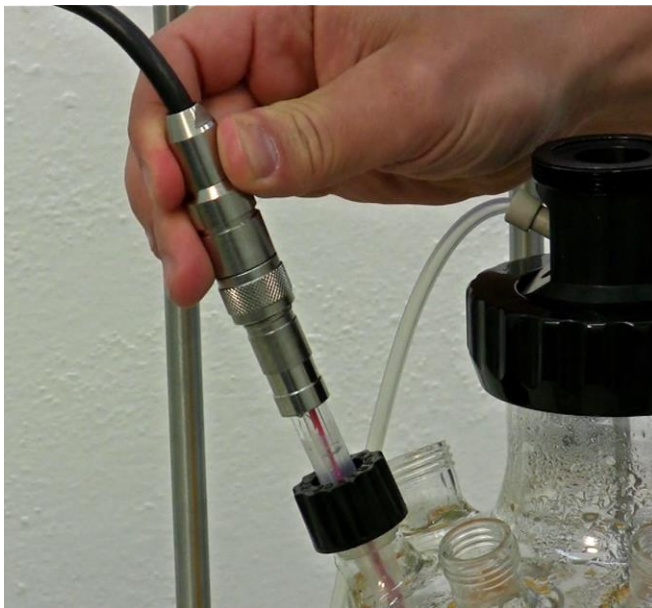
Figure 3.8—11 Connect the pH probe connector (black) cable from the MINIFOR base control unit with the pH probe. Rotate and adjust the connector cable for exact locking of grooves.
