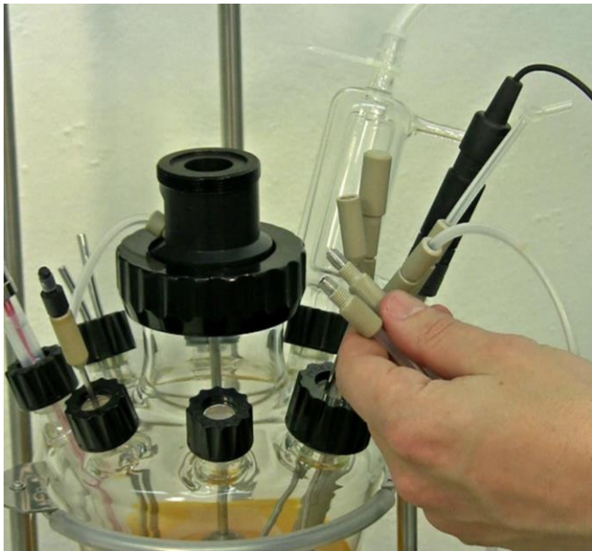
Figure 3.10—27 Take the prepared tubing with the PEEK double-seal tubing connectors at both the ends of the tubing (Refer 10.3.2 Preparation of PEEK double-seal tubing connectors).
