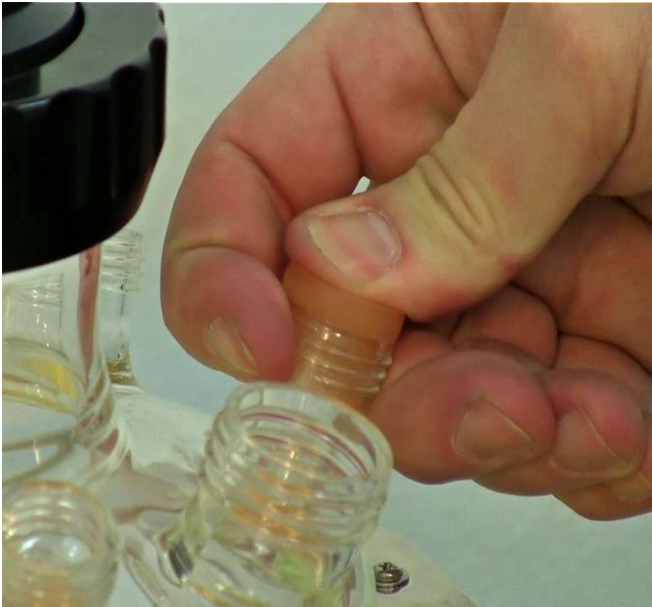
Figure 3.7—5 Insert the coloured rubber stopper for the pO 2 (DO) probe on the right side of the port which is next to the sampling port (larger in diameter)
