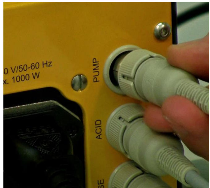
Figure 3.16—19 Other additional pumps can be connected to the PUMP socket.
