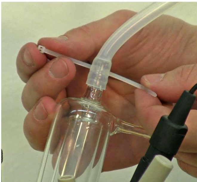
Figure 3.12—4 Seal the tubing with the “locking strap” as shown. It is recommended to place a small piece of vertically cut tubing above this before sealing with the “locking strap”.
