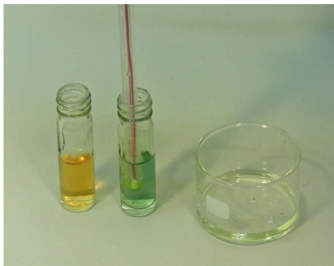
Figure 5.2—19 Test the measurement of the pH into, by dipping the probe into the pH 7 buffer solution.
