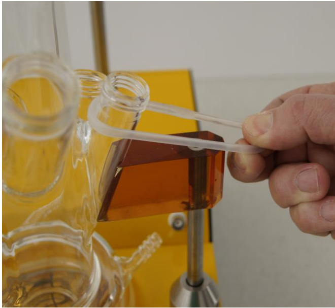
Figure 3.4—17 Place the elastic silicone ring on the distinct side arms of the pH and pO 2 probe.
