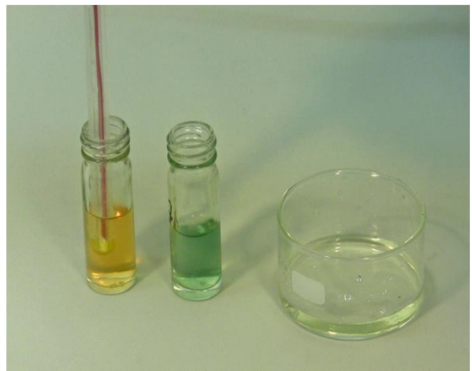
Figure 5.2—6 Dip the probe into the gauging solution (pH 4 buffer solution) and stir gently while the pH is being measured.
