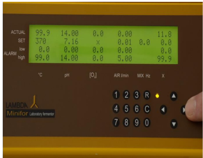
Figure 4.3—2 Enter the value for the desired temperature (the value shown on the first line and first column corresponds to the measured temperature and cannot be changed).
