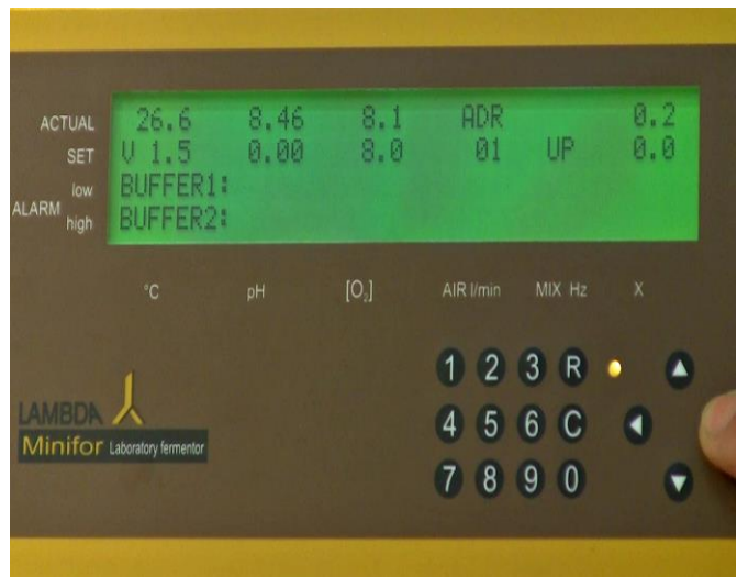
Figure 5.3—6 Once right arrow key is pressed, the value will be saved. (e.g.: 8.0)
