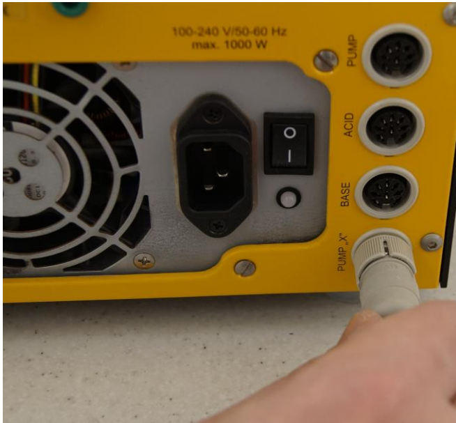
Figure 3.13—8 Connect the corresponding pump to the “PUMP X” *) socket on the rear of fermentor-bioreactor MINIFOR.
