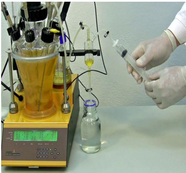
Figure 8.2—3 Pull the plunger of the syringe to fill the sampling glass device with the sample from the reaction vessel. Never fill the glass device completely.
