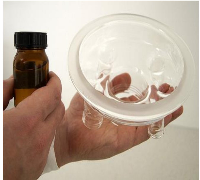
Figure 3.4—26 Apply a small amount of silicone oil on the vessel upper part's brim for easy removal of the parts after completing the experiment.
