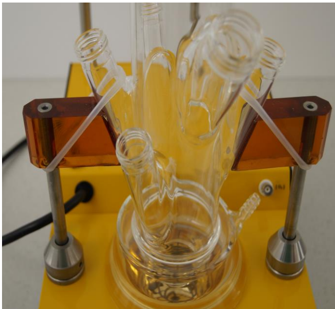
Figure 3.4—19 The reaction vessel mounted on the base unit and made intact with the help of the lateral holder and elastic silicone ring.
