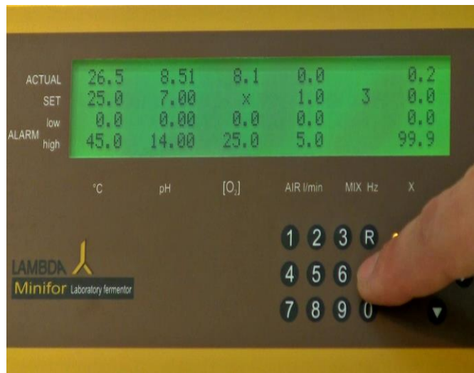
Figure 4.1—2 “C” - Calibration key is pressed to change the stand-by mode to calibration mode.
