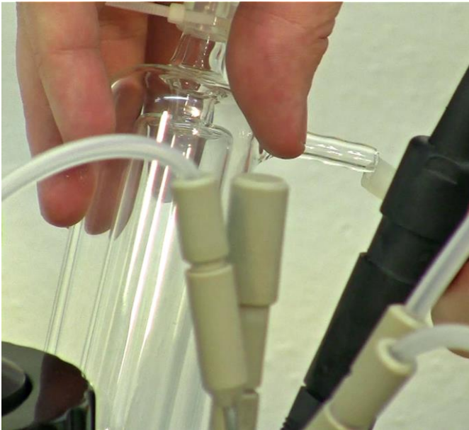
Figure 3.12—5 Connect the cooling water to the outgas condenser. (Lower arm = inlet, Upper arm = outlet for cooling water).
