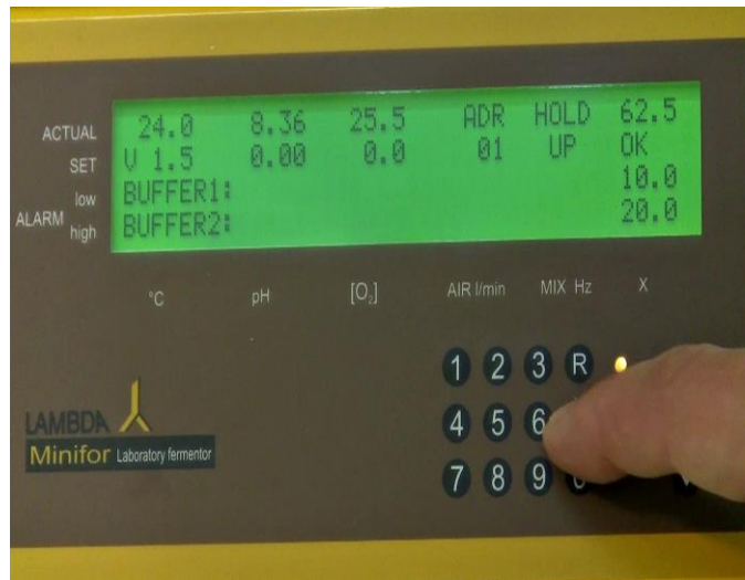
Figure 5.5—12 Wait until the message “HOLD” appears and then press the calibration key “C”. The message “OK” will appear indicating that the calibration has been accepted by the MINIFOR fermentor unit. Now, the scale is calibrated in g or ml. Weight calibrations can be made according to your need with weights.
