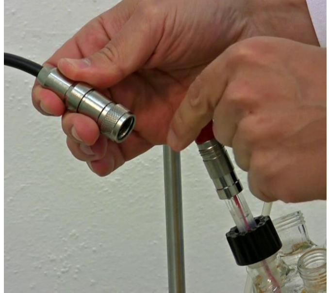
Figure 3.15—6 Remove the protective cap from the pH probe (red cap)
