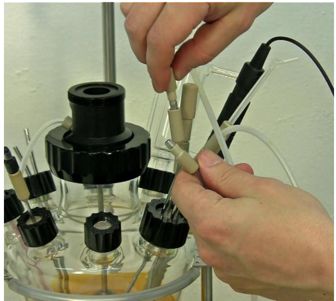
Figure 3.10—28 Connect one end of the prepared tubing with the PEEK double seal tubing connector to the short cannula in the quadruple sampling port.
