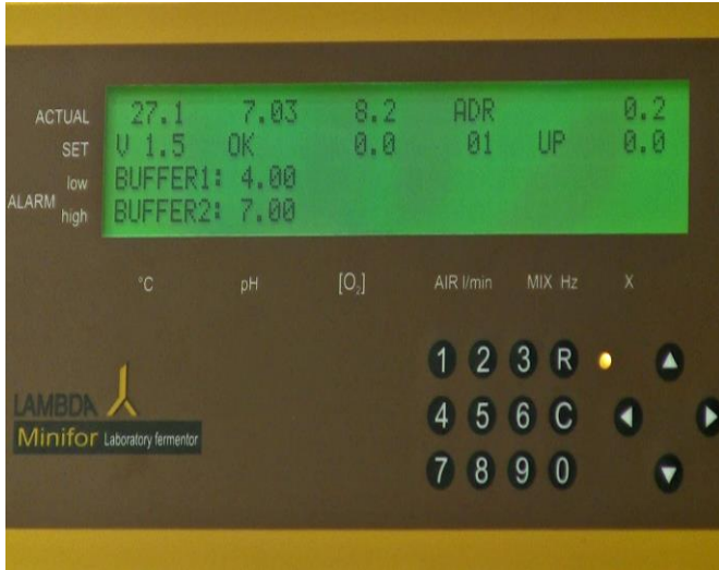
Figure 5.2—15 OK message will be displayed, if the calibration is done correctly.
